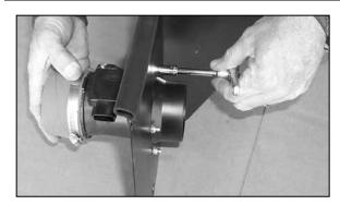
28. Install the silicone hose (084031) and hose clamp #56 onto the mass air sensor then assemble the mass air sensor and filter adapter onto the heat shield using the supplied hardware, 4 -washers, 4 - 25mm bolts and 4 - nylock nuts.
