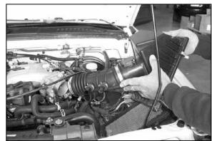
9. Unlatch the four clips on the air filter housing and remove the top assembly.
