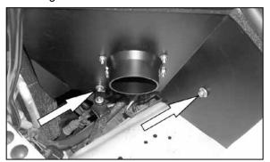
30. Align holes with brackets and attach using hardware provided. Do not tighten completely. **NOTE: brackets go on engine side of heat shield.**
