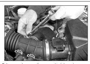
7. Loosen clamp on the resonator tube using a 10mm socket.
