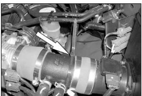
36. Using the zip-tie removed in step 3, secure the mass air sensor electrical connection to the K&N® intake tube as shown.
