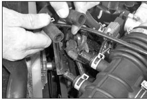
5. Remove the two hoses from the intake tube.
