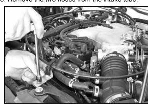
6. Disconnect the cruise control cable bracket using a 10mm socket.
