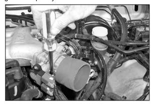
25. Install silicone hose, (08096), and hose clamp #44 onto the throttle body and tighten.
