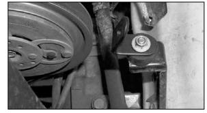
24. Attach the bracket, 070004, onto the front rubber mount, #2,(see picture on step #22). Do not tighten completely at this time.
