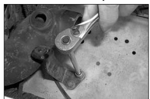
14. Remove the front support bracket using a 10mm socket.
