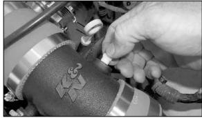
32. On vehicles **NOT** equipped with a map / baro switch solenoid valve, install the provided plug, (08178) onto the intake tube.
