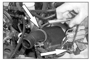
17. Remove the two bolts on rear resonator box using a 10mm socket.
