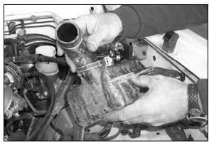
19. Remove the resonator box as shown.
