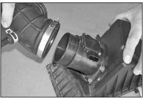
20. Loosen hose clamp using an 10mm socket and remove air duct tube from mass air sensor.
