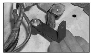
23. Attach slotted end of bracket, 070662, onto rubber mount, #1, (see picture on step #22), with washer and lock nut. Do not tighten completely.
