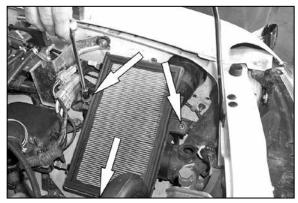
12. Remove the three bolts that secure the lower air filter housing using an 8mm socket.
