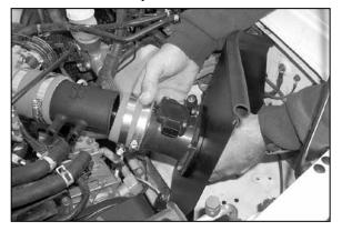
29. Install heat shield assembly, using hose clamp #48 sliding over intake tube.
