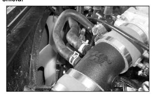
31. Align intake tube for best fit then tighten hose clamps. Reattach the two hoses onto the intake tube.
