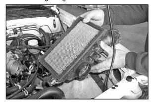
13. Remove the lower air filter housing as shown NOTE: K&N Engineering, Inc., recommends that customers do not discard factory air intake.
