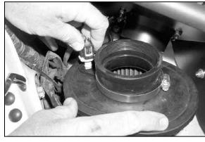
38. Insert air temp sensor into base of air filter.
