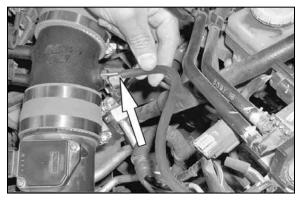
33. On vehicles equipped with a map/baro switch solenoid valve, install vent (087016) and attach hose to the intake tube.
