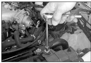
15. Remove bolt from front of resonator using a 10mm socket.
