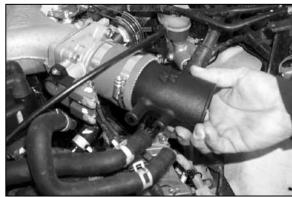
26. Install hose clamp #48 and the intake tube onto the silicone hose on the throttle body. Do not tighten completely.
