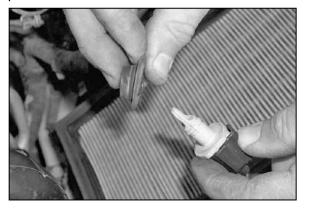
11. Remove rubber grommet from air temp sensor.
