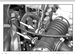
4. Squeeze the two hose clamps and slide back using pliers.
