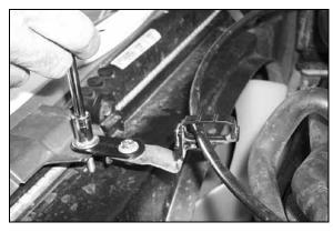
37. Reconnect the throttle cable bracket using the flat bracket, two washers, 10mm bolt, nylock nut and the stock bolt. Tighten completely.
