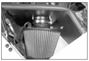
39. Install RX-4750 air filter element and secure with hose clamp using an 8mm socket or nut driver. NOTE: Drycharger® air filter wrap; part # RF-1042DK is available to purchase separately. To learn more about Drycharger® filter wraps or look up color availability please visit http://www.knfilters.com®.
