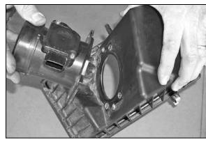
21. Remove the four bolts from mass air sensor housing using a 10mm socket and detach from airbox.
