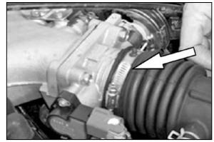
8. Loosen clamp at the throttle body using an 8mm socket.
