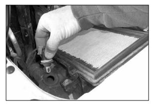
10. Remove the air temp sensor by pulling in an upward direction as shown.
