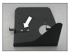
9. Install the heat shield mounting bracket (083126) onto the heat shield and secure with the provided hardware.
