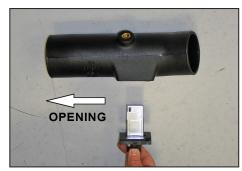
19. Install the mass air sensor assembly into the  $K\&N^{\otimes}$  intake tube as shown and secure with the provided hardware.
