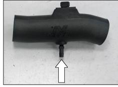
20. Install the provided vent fitting into the  $K\&N^{\otimes}$  intake tube as shown.
