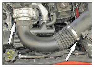
4. Loosen the intake tube mounting clamps and then remove the factory intake tube from the vehicle.
