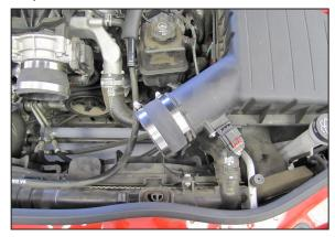
9. Install the remaining coupling hose onto the air box outlet and secure with the provided hose clamps.
