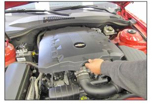
2. Remove the oil fill cap and then lift up the engine cover and remove it from the engine. Reinstall the oil fill cap at this time.
