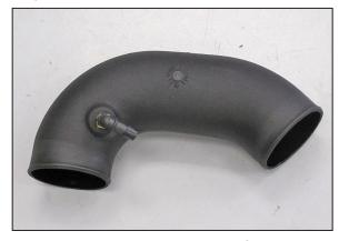
10. Install the 90° fitting into the K&N $^{\mbox{\tiny \$}}$  intake tube as shown.
