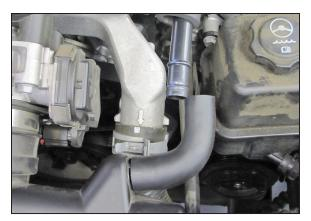
3. Disconnect the Crank case vent hose from the crank case vent tube.
