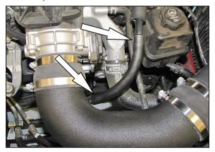
12. Connect the provided crank case breather hose onto the fitting installed into the K&N<sup>®</sup> intake tube and then attach the open end to the factory crank case vent tube.
