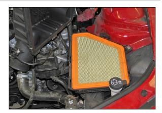
5. Releases the upper air box cover latches' and lift off the upper air box, then remove the factory air
