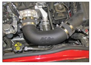
11. Install the K&N<sup>®</sup> intake tube into the coupling hose on the air box and then into the hose on the throttle body. Secure the tube with the provided hose clamps.
