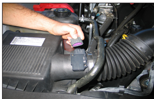
2. Disconnect the mass air sensor electrical connection.
