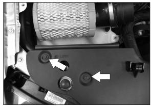
9. Reinstall the retaining clip and bolt removed in step #6 to secure the core support cover.
