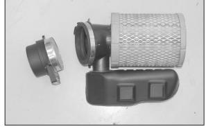
11. Loosen the hose clamp, which secures the mass air sensor to the filter assembly, and then remove the mass air sensor as shown.
