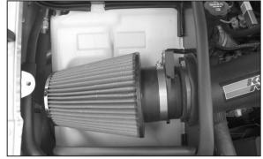
29. Install the K&N<sup>®</sup> Air Filter onto the mass air sensor and secure with the provided hose clamp as shown.
