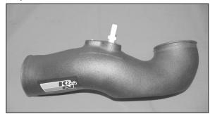
23. Install the provided vent fitting into the intake tube as shown.
