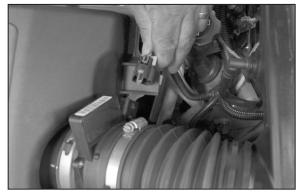
3. Depress the locking tab on the mass air sensor electrical connection and then separate the connector from the mass air sensor.
