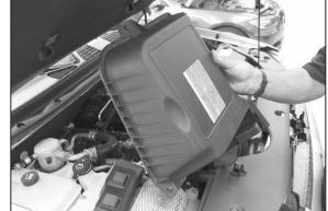
2. Remove the wing nut, which retains the engine cover and then remove the engine cover.
