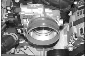
22. Install the silicone hose (08755) onto the throttle body and secure with the provided hose clamp as shown.
