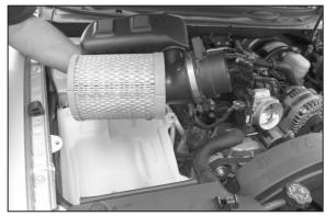
10. Remove the filter and mass air sensor assembly from the vehicle as shown.
