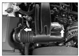
4. Loosen the two hose clamps, which secure the intake tube to the mass air sensor and throttle body.
