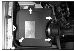
7. Loosen the four airbox lid retaining bolts shown.
