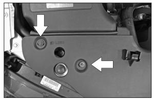
6. Remove the core support cover bolt and retaining clip shown.
