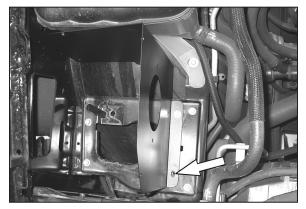
11a. On vehicles that are not equipped with the front airbox mounting grommet and hole, install the heat shield assembly as shown. Then, use a marker to mark the mounting plate through the heat shield mounting hole.
