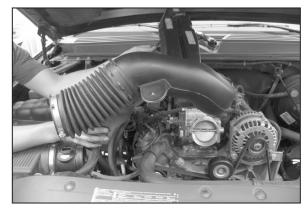
6. Loosen the hose clamps, which secure stock intake tube to the throttle body and mass air sensor and then remove the intake tube from the vehicle.
