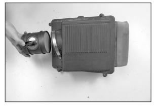
8. Loosen the hose clamp and remove the mass air sensor from the air cleaner as shown.
