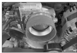
16. Install the silicone (08631) hose onto the throttle body and secure with the provided hose clamp.
