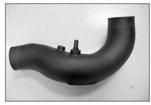
18. Install the NPT fitting into the  $K\&N^{\tiny \$}$  intake tube as shown.
