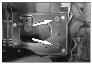
12. Install the two 5/16" inserted nuts into the airbox mounting tray as shown.
