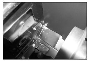
14. Secure the heat shield mounting bracket to the inner fender with the fender washers and hardware as shown.
