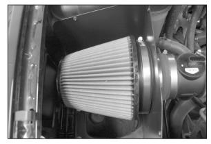
24. Install the K&N® air filter as shown and secure with the provided hose clamp.
