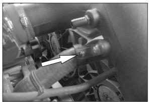
22. Install the upper radiator hose mount onto the mounting bracket installed onto the K&N® intake tube and secure with the provided tie wrap as shown.
