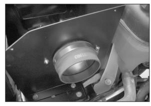
15. Install the silicone hose (08618) onto the filter adapter and secure with the provided hose clamp.
