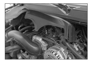
3. Lift up on the front of the engine cover to diengage from the mounting grommets. Then pull forward and remove the engine cover from the engine as shown.
