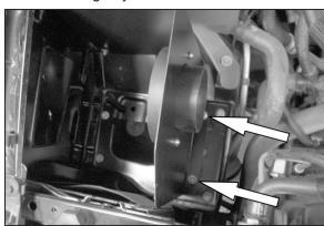
13. Install the heat shield assembly onto the airbox mounting tray and secure to the 5/16" inserted nuts with the provided hardware as shown.
