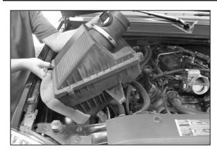
7. Pull firmly upwards to release the air cleaner assembly from the mounting tray grommets, and then remove the assembly as shown.
