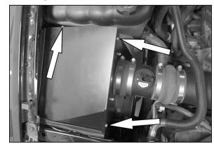
26. Install the filter cover onto the heat shield and secure with the provided hardware.
