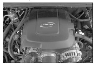
27. Re-install the engine cover removed in step #3.
