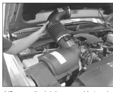
4. Lift up on the intake assembly to release from the mounting grommets and then remove the assembly from the vehicle as shown.
