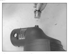
9. Remove the air filter restriction gauge and stock grommet from the air filter housing as shown.
