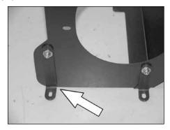
14. Install the "L" bracket (070952) onto the heat shield as shown with the provided hardware as shown.
