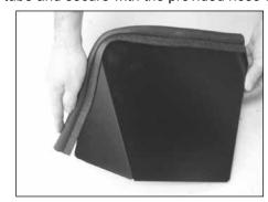
21. Install the edge trim onto the heat shield lid as shown.
