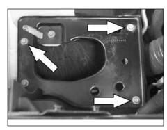
7. Remove the three bolts shown which secure the mounting plate.
