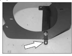
13. Install the "L" bracket (07805) onto the heat shield as shown with the provided hardware as shown.
