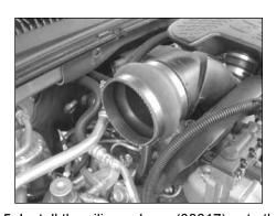
5. Install the silicone hose (08617) onto the intake manifold and secure with the provided hose clamp as shown.
