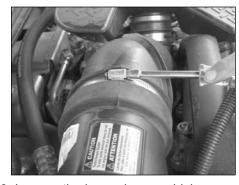
3. Loosen the hose clamps which secure the intake tube to the intake manifold and air box, then remove the intake tube from the vehicle.
