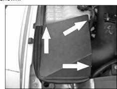
22. Install the heat shield lid onto the heat shield and secure with the three 5mm button head allen bolts provided.
