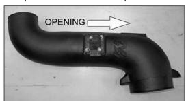
11a. Install the mass air sensor assembly into the  $K\&N^{\odot}$  intake tube and secure with the provided hardware.
