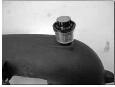
12. Install the factory grommet and filter restriction gauge into the K&N® intake tube as shown.
