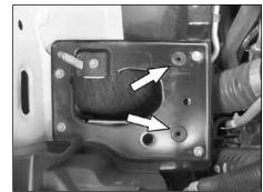
6. Remove the two mounting grommets shown from the mounting plate.
