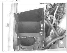
17. Install the heat shield onto the air box mounting plate and secure with the factory bolts removed in step #7.
