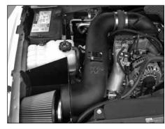
19. Secure the K&N® intake tube to the silicone hose at the throttle body with the hose clamp provided and to the heat shield with the provided hardware.
