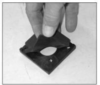
10.Attach the provided gasket onto the back of the K&N® mass air adapter as shown.
