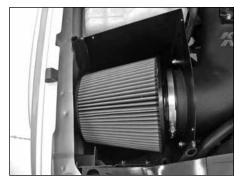
20. Install the K&N® air filter onto the K&N® intake tube and secure with the provided hose clamp.
