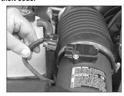
2. Depress the locking tab on the mass air sensor electrical connector, and then disconnect the electrical connection as shown.
