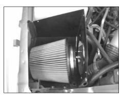
18. Set the  $K\&N^{\otimes}$  air filter into the heat shield as shown.
