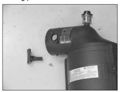
8. Using the "TORX" T20 wrench, remove the two bolts, which secure the mass air sensor to the air filter housing and then remove the mass air sensor.
