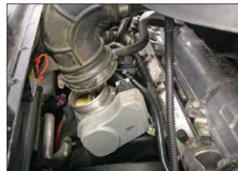
3. Loosen the hose clamp, which secures the intake tube to the throttle body, and then pull up on the intake tube/airbox assembly to dislodge it from the mounting grommets and disconnect the intake tube from the throttle body.
