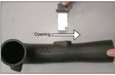
8. Install the mass air sensor into the intake tube as
