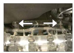
11. Remove the two stock airbox mounting anchors shown from the mounting bracket.
