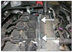
13. Thread and tighten the two coupling nuts onto the studs installed in step #12.
