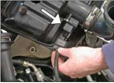
5. Flip the airbox assembly up towards the driver's side of the vehicle to gain access to the mass air sensor electrical connection, and then disconnect the mass air sensor electrical connection as shown.
