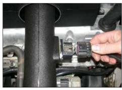
22. Reconnect the vehicles mass air sensor electrical connection.
