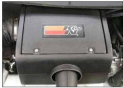
21. Install the K&N® airbox lid and secure with the provided hardware as shown.
