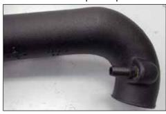
10. Install the supplied crankcase vent fitting into the intake tube as shown.
