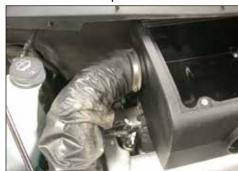
15. Install the fresh air supply hose onto the K&N® airbox and secure with the factory hose clamp.
