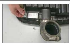
7. Remove the two screws securing the mass air sensor to the stock intake tube and then remove the sensor as shown.
