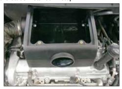
14. Install the K&N® airbox onto the engine. Using the supplied hardware, secure the airbox to the rear mounting bracket first and then to the coupling nuts installed in step #13.
