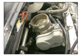
16. Install the silicone hose (08756) onto the throttle body and secure with the provided hose clamp.
