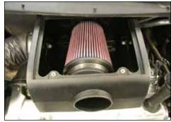
18. Place the filter assembly into the K&N® airbox as shown.
