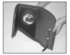
12. Install the edge trim onto the inner hole on the heat shield as shown. Trim if needed.
