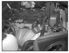
21. Install the tube-mounting bracket assembly onto the resonator-mounting tab on the valve cover with the provided hardware as shown.
