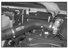
22. Install the K&N<sup>®</sup> intake tube into the silicone hose at the throttle body and through the heat shield so it rests onto the tube-mounting bracket assembly, then secure with the provided hose clamps.
