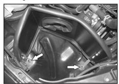
14. Install the heat shield into the vehicle using the hardware provided and the factory airbox retaining nut.
