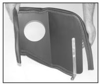
11. Install the edge trim onto the heat shield as shown.
