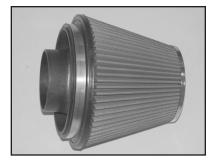
25. Install the filter adapter into the K&N<sup>®</sup> air filter and secure with the provided hose clamp. NOTE: Drycharger<sup>®</sup> air filter wrap; part # RF-1048DK is available to purchase separately. To learn more about Drycharger<sup>®</sup> filter wraps or look up color availability please visit http:// www.knfilters.com<sup>®</sup>.
