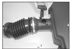
15. Remove the mass air sensor from the stock airbox as shown.
