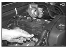
19. Remove the clip nut from the forward resonator mount on the valve cover as shown.
