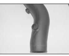
18a. On vehicles not equipped with a fuel pressure regulator vent hose, install the provided NPT plug into the K&N<sup>®</sup> intake tube as shown.
