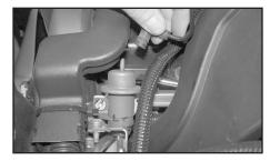
6. On vehicles equipped with a fuel pressure regulator disconnect the fuel pressure regulator vacuum hose from the fuel pressure regulator as shown.
