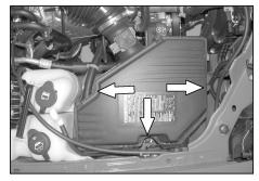
4. Loosen the two airbox retaining bolts and one retaining nut.
