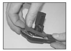
16. Apply provided gasket to mass air sensor as shown.
