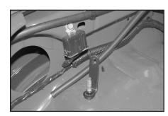
13. Install the "L" bracket (070602) onto the stock airbox mounting stud using the factory airbox retaining nut.
