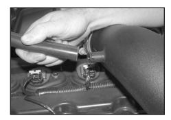
24. Install the provided crankcase vent hose onto the valve cover, then onto the K&N $^{\circ}$  intake tube as shown.
