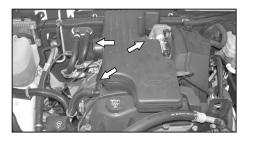
7. Loosen the two bolts that retain the intake resonator to the engine, and then loosen the hose clamp at the throttle body.
