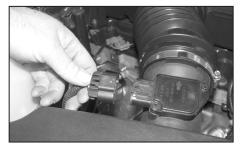
2. Depress the locking clip on the mass air sensor electrical connection, and then separate the mass air sensor electrical connection. 3. Loosen the hose clamp that retains the stock intake tube to the resonator, and then remove the tube from the resonator as shown.
