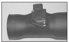
17. Install the mass air sensor assembly into the  $K\&N^{\odot}$  intake tube using the provided spacers and button head allen bolts provided.
