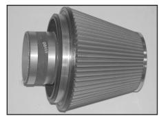
26. Install the silicone hose (08630) onto the air filter assembly as shown.
