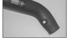
18. Install the provided  $\frac{1}{4}$ " NPT vacuum fitting into the K&N<sup>®</sup> intake tube as shown.
