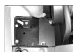
13. Adjust the heat shield and intake tube for best fit, then tighten the two hex bolts as shown.
