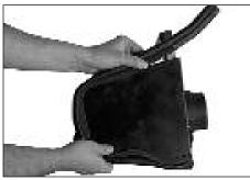
8. Apply the trim seal to the heat shield assembly as shown.
