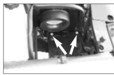
9. Install and mount the heat shield assembly to the air cleaner mounting tray using the bolts removed in step 5.
