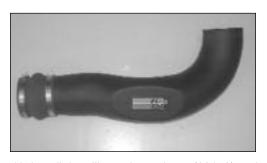
11. Install the silicone hump hose (08176) and hose clamps onto the K&N intake tube as shown.
