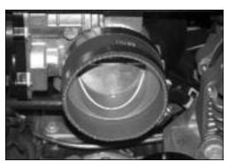
10. Install the silicone hose (08625) and hose clamps onto the throttle body as shown.
