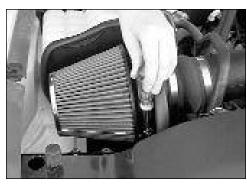
14. Install the K&N air filter onto the heat shield assembly as shown.
