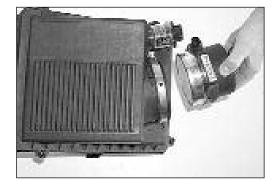
6. Loosen the hose clamp and remove the mass air sensor from the air cleaner.
