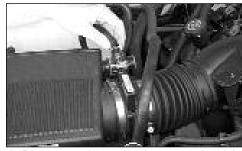
2. Disconnect the mass air sensor electrician connection.
