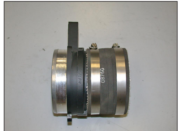
18. Install the provided silicone hose (08631) onto the mass air sensor and secure with the provided hose clamp as shown.
