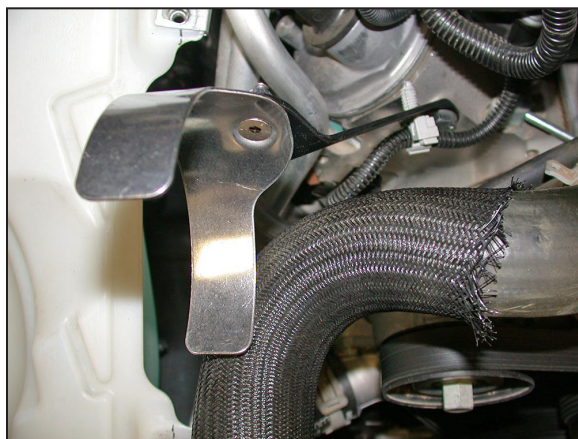
14. Install the wiring harness retaining clip removed in step #11 into the new tube mounting bracket, and then resecure the wire harness to the clip as shown.
