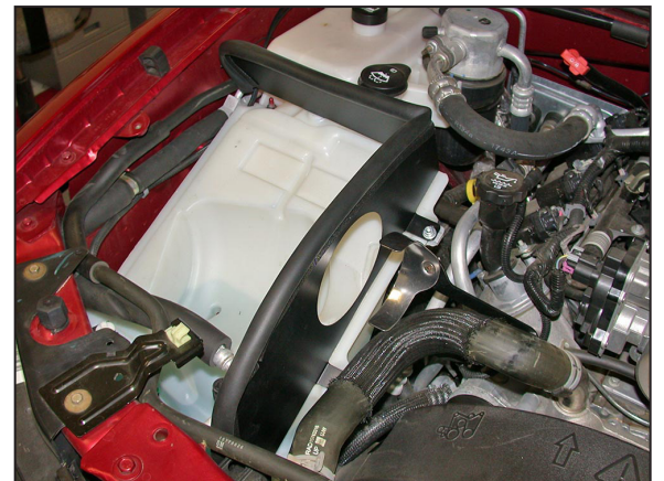
16. Install the heat shield assembly into the vehicle using the provided hardware.
