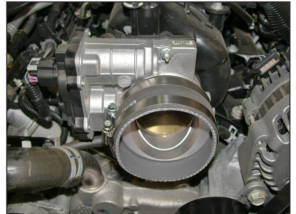
17. Install the provided silicone hose (08625) onto the throttle body and secure with the provided hose clamp as shown.
