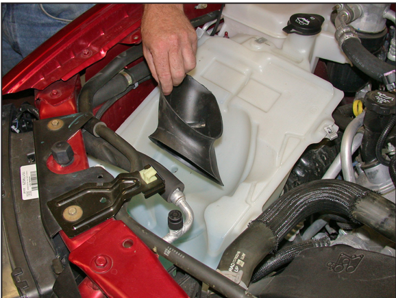
9. Remove the fresh air supply tube from the lower air box / washer reservoir housing.
