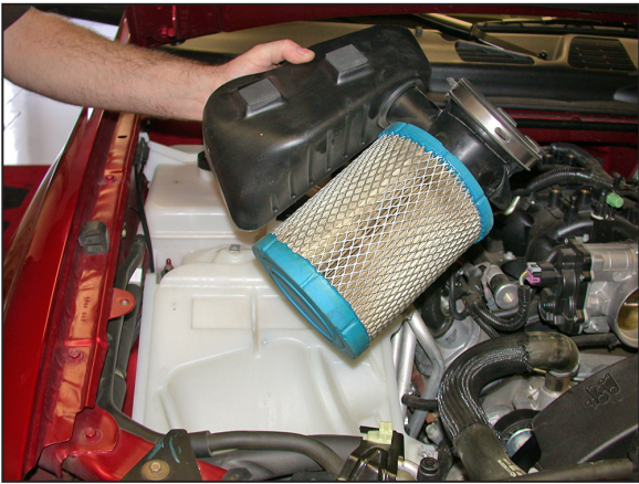
8. Remove the stock air filter assembly from the vehicle as shown. NOTE: K&N Engineering, Inc., recommends that customers do not discard factory air intake.
