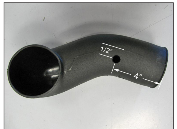
18a. On vehicles equipped with a crank case vent, mark the tube 4" back from the end of the tube and 1/2" below the mold seam then drill a 5/8" id hole.
