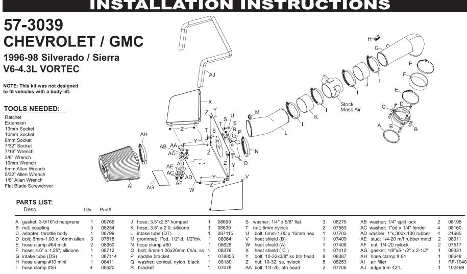
NOTE: FAILURE TO FOLLOW INSTALLATION INSTRUCTIONS AND NOT USING THE PROVIDED HARDWARE MAY DAMAGE THE INTAKE TUBE, THROTTLE BODY, AND ENGINE.
