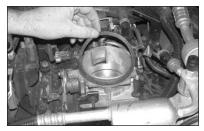
16. Install the neoprene gasket provided onto the throttle body flange.
