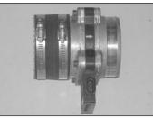
30. Install the silicone hose (08630) onto the mass air sensor inlet side.
