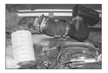
7. Lift and remove the complete air intake system.
