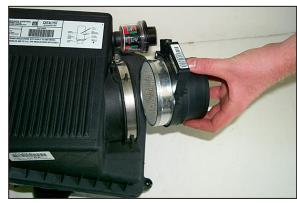
6. Loosen the hose clamp and remove the mass air sensor from the air cleaner.
