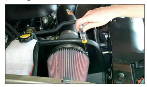
16. Install the K&N® Air Filter onto the heat shield assembly as shown.
