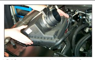
4 Pull firmly upwards to release the airbox from the factory grommets, then remove the factory air cleaner as shown.
