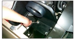
15. Adjust the heat shield and intake tube for best fit, then tighten the two hex bolts as shown.
