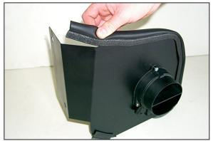
8. Apply the trim seal to the heat shield assembly as shown.
