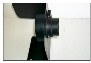
7. Assemble the mass air adapter, heat shield, gaskets and the mass air sensor as shown above.
