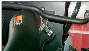
17. Reconnect the mass air sensor electrical connection as shown.
