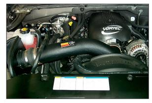
14. Install the K&N® intake tube onto the mass air sensor, then secure the other end onto the throttle body as shown.
