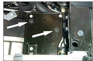
9. Install the two provided nut-serts into the air cleaner tray as shown. See arrows.
