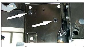
5 Remove the two factory grommets from the stock air cleaner tray as shown. See arrows.
