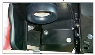
11. Using the provided hardware, secure the heat shield assembly to the nut-serts as shown. NOTE: finger tighten the bolts as some adjustment may be necessary.
