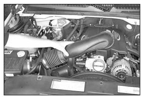
3. Loosen the hose clamps at the throttle body and at the mass air sensor, then remove the factory intake tube.
