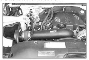
12. Slide the K&N® intake into the hump hose at the mass air sensor, then slide the tube into the silicone hose at the throttle body and tighten the hose clamps.
