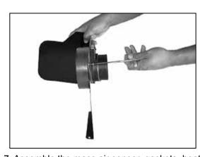
7. Assemble the mass air sensor, gaskets, heat shield and mass air adapter with the provided hardware as shown.
