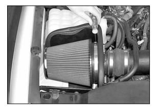
13. Install the K&N® air filter onto the mass air adapter and secure it with the provided hose clamp.
