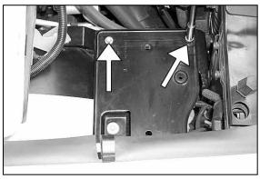
5. Loosen and remove the two air cleaner mounting tray bolts as shown.
