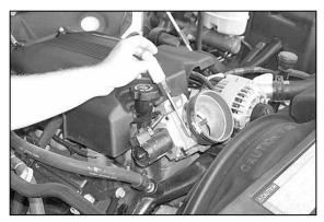
10. Install the silicone hose and hose clamps onto the throttle body as shown.
