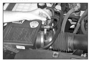
2. Disconnect the vehicle's mass air sensor.
