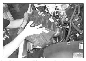
4. Pull firmly upward to release the air cleaner from it's mounting grommets, then remove the air cleaner assembly.
