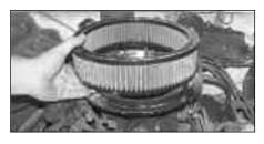
8. Install the K&N Filtercharger onto the base plate as shown.
