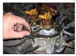
7. Remove the factory air cleaner gasket.
