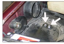
5a. On vehicles equipped with rear A/C-heat, secure the heater hose manifold bracket to the inner fender with the factory bolts removed in step #5 and the nuts provided.
