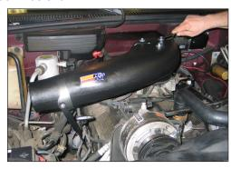
17. Re-install the K&N® intake tube and secure it with the provided washers and nylock nuts.
