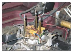
13. Apply the three nylock nuts onto the throttle body studs as shown approximately 3/4" down.
