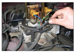
16. Remove the paper backing from the gasket and apply the gasket to the throttle body sticky side down as shown.
