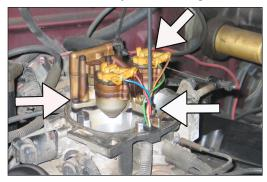
8. Remove the three factory Torx screws from the throttle body assembly.
