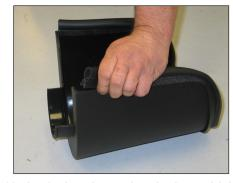
19. Apply the trim seal to the heat shield as shown.
