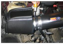
20. Install the heat shield onto the tube as shown, but do not tighten completely.
