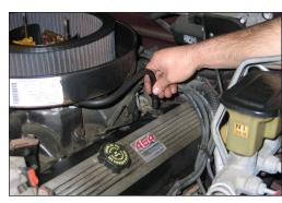
3. Remove the crank case vent line from the valve cover.
