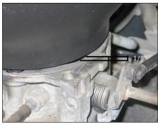
15. Install the K&N® intake tube onto the throttle body.
