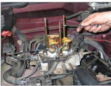
9. Install the three provided throttle body studs into the three holes from step 8.
