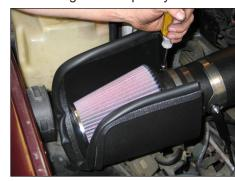
21. Install the K&N® air filter onto the intake tube as shown.
