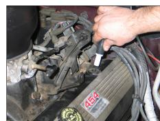
23. Attach the silicon hose onto the vent on the intake tube, then, push the hose mender into the grommet in the valve cover.
