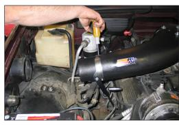
18. Secure the tube to the saddle bracket assembly using the provided hose clamp.
