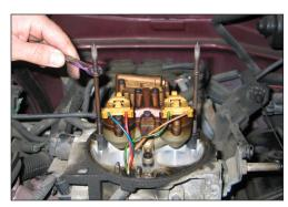
6a. On 92-95 vehicles, remove the two factory throttle body studs as shown.
