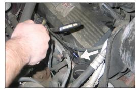
11. Loosen and remove the valve cover bolt as shown .
