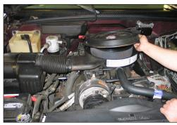
2. Loosen and remove the air cleaner wing nuts, then remove the air cleaner lid.
