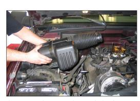
5. Loosen and remove the two bolts that secure the air inlet/resonator, then, remove the complete assembly.
