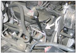
12. Secure the saddle bracket assembly to the valve cover using the bolt removed in step 11. Do not tighten completely.
