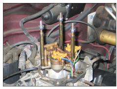
14. Apply the 1/4" washers onto the studs as shown above.
