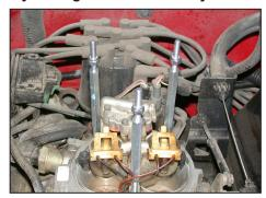
10. Install the three provided nylock nuts onto the throttle body studs approximately 3/4" down as shown.
