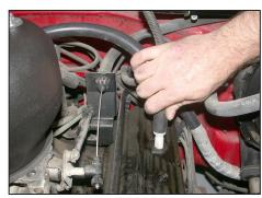
24. Install the silicone hose onto the vent on the K&N® intake tube, then push the hose mender into the grommet on the valve cover.
