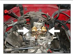
7a. On 92-95 vehicles, remove the two factory throttle body studs as shown.
