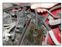
5. Remove the crank case vent line from the valve cover as shown.
