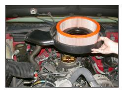
3. Disconnect the cold inlet tube and then remove the air cleaner base assebmly as shown.
