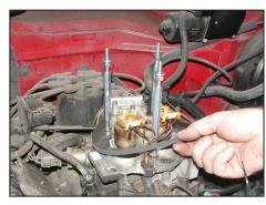
18. Remove the paper backing from the provided gasket and install the gasket onto the throttle body sticky side down.
