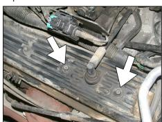
15. Remove the two valve cover bolts as shown.
