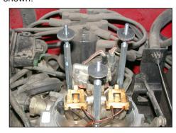
11. Install the three flat washers onto the throttle body studs as shown.
