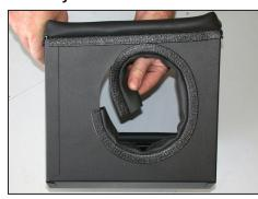
13. Install the short piece of trim seal to the heat shield as shown.
