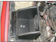
14. Install the heat shield to the inner fender using the provided hardware as shown.
