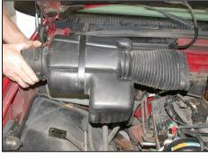
4. Loosen and remove the two bolts that secure the air inlet/resonator, then remove the assembly as shown.
