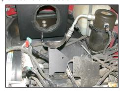
17. Install the saddle bracket assembly using the two bolts removed in step 15.
