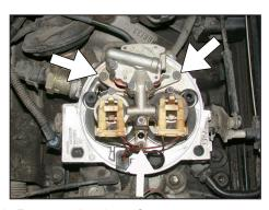
8. Remove the three factory torx screws as shown.
