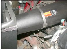
21. Secure the K&N® intake tube to the saddle bracket assembly with the provided hose clamp.
