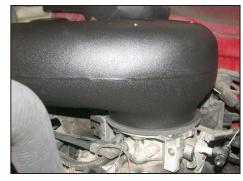
19. Install the K&N® intake tube onto the throttle body.
