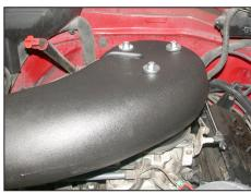
20. Reinstall the K&N® intake tube and secure it with the provided washers and nylock nuts.
