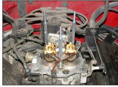
9. Install the three provided throttle body studs into the three holes from step 8.
