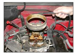
6. Remove the throttle body spacer as shown.
