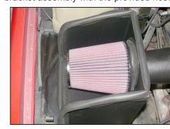
22. Install the K&N $^{\! \rm 8}$  air filter onto the K&N $^{\! \rm 8}$  intake tube as shown.
