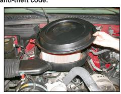
2. Loosen and remove the air cleaner wing nuts, then remove the air cleaner lid.
