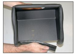
12. Install the long piece of trim seal onto the heat shield as shown.
