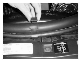
3. Detach the clip that retains the a/c lines to the radiator shroud.
