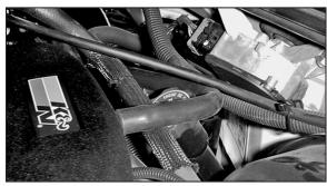
33. Attach the vent hose to the vent fitting on the intake tube.
