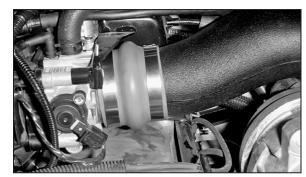
31. Attach the hump hose to the throttle body and tighten hose clamp.
