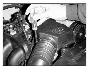
5. Loosen the hose clamp on the intake hose at the resonator.
