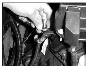
17. Install the 3/8"ID grommet onto the airbox mounting stud.
