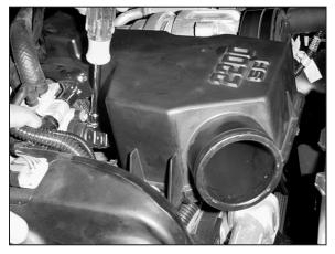
13. Loosen the hose clamp on the resonator at the throttle body.
