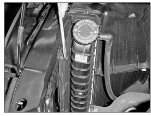
18. Pry up on and remove the two push clips from the radiator core support.
