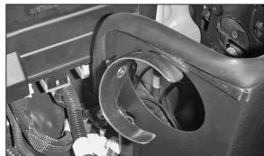
22. Install the saddle bracket assembly onto the airbox mounting stud and secure using the hardware provided.
