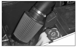
34. Install the Air Filter and tighten hose clamp.
