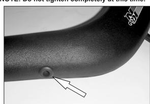
23. Install the 1/2"ID grommet into the K&N $^{\! \rm 8}$  intake tube.
