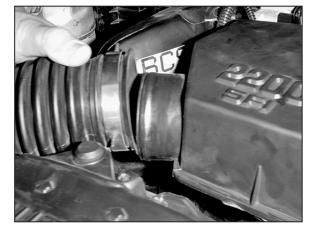
7. Detach the intake hose from the resonator.
