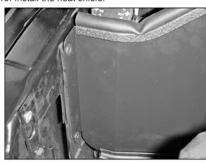
20. Secure the heat shield to the radiator core support using the clips removed in step 18.
