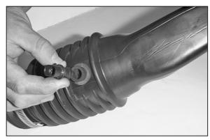
24. Remove the air temperature sensor from the stock intake hose.
