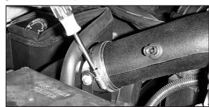
32. Secure the saddle bracket to the intake tube using the hose clamp provided.
