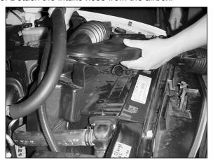
9. Remove the entire intake tube assembly.
