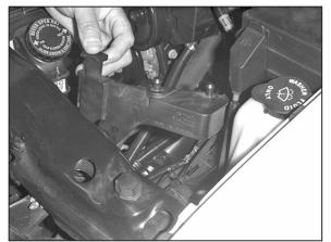
11. Press on the tab and lift and remove the airbox mounting bracket from the radiator core support.
