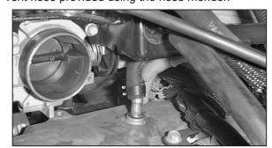
29. Attach the vent hose assembly to the vent fitting on the valve cover.
