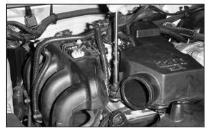
12. Loosen and remove the bolt that retains the resonator to it's mounting bracket.
