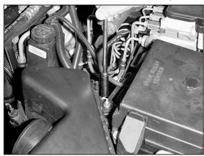
10. Loosen and remove the nut that retains the airbox to its mounting stud and remove airbox.
