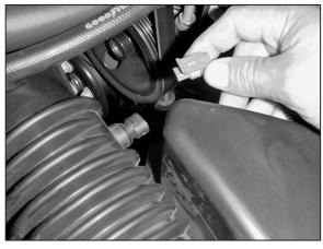
2. Disconnect the air temperature sensor electrical connection.
