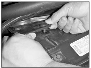
6. Pry up on the two push clips that retain the intake tube to the radiator shroud.
