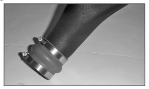
26. Attach the hump hose onto the K&N® intake tube and tighten hose clamp.
