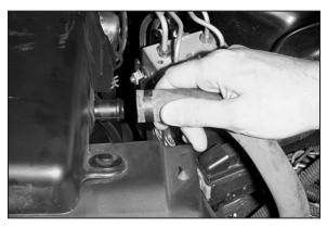
4. On models equipped with air injection, detach the air injection hose from the resonator.
