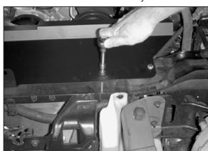
13. Secure the heat shield to the radiator core support using the hardware provided.
