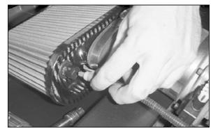
32. Reconnect the air temperature sensor electrical connection.
