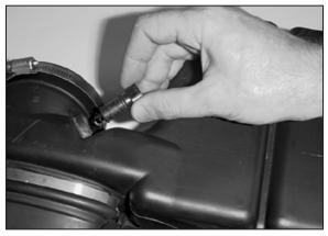
16. Remove the air temp sensor from the resonator.
