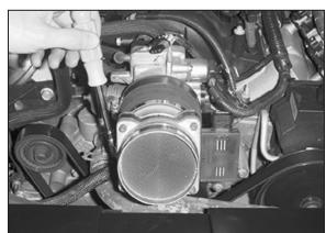
18. Install the mass air sensor into the silicone hose and tighten hose clamp.
