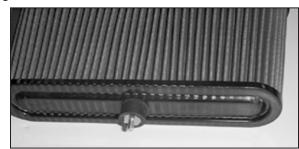
21. Install the rubber mounted stud into the threaded hole on the top plate of the filter.
