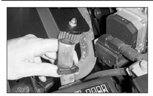
29. On models with air injection, cut the air injection vent hose at the mark.
