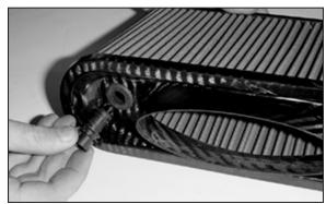
20. Insert the air temp sensor into the grommet.
