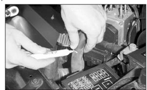
28. On models with air injection, align the air injection vent hose with the flange of the vent filter and mark.
