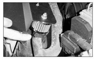
30. On models with air injection, attach the air injection hose to the flange on the vent filter using the O.E. clamp.
