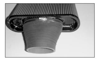
22. Attach the round oval silicone hose on to the flange of the filter.
