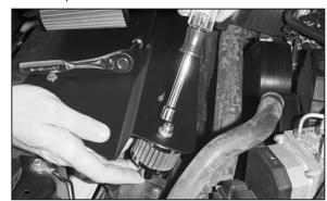
27. On models equipped with air injection, attach the vent filter to the heat shield using the hardware provided.
