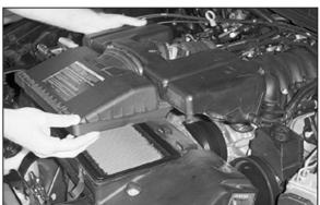
8. Detach the intake hose from the throttle body and remove the entire upper air intake assembly.
