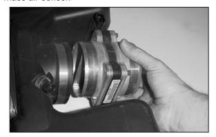
15. Loosen the hose clamp on the flange of the air box and remove the mass air sensor.
