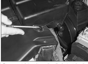
5. Pry up on tab to release the clip that retains the resonator to the radiator cover.
