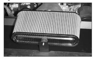
23. Install the air filter assembly attaching the silicone hose to the mass air sensor.
