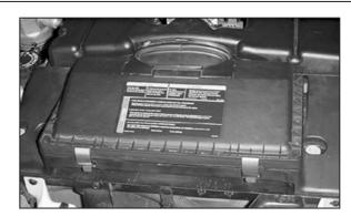
7. Release the two clips that retain the air box top to the air box base.
