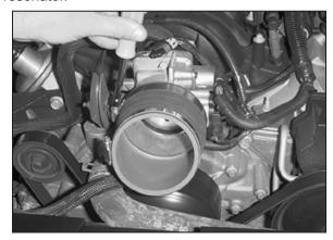
17. Attach the silicone hose to the throttle body. Note: Do not tighten the hose clamp completely at this time.
