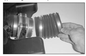
14. Loosen the hose clamp on the intake hose at the mass air sensor then detach the hose from the mass air sensor.
