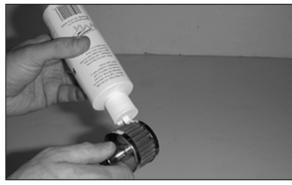
26. On models equipped with air injection, oil the vent filter provided.
