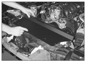
12. Install the heat shield assembly.
