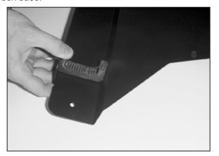
11. Install the rubber cushions onto the heat shield as shown.
