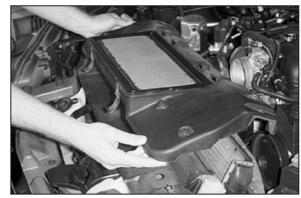
9. Loosen and remove the 4 bolts that retain the air box base to the radiator core support, then remove the lower air box assembly.
