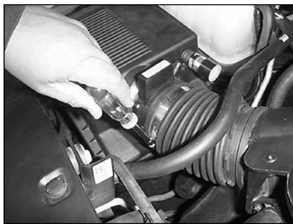
3. Loosen the hose clamp on the intake hose at the mass air sensor.
