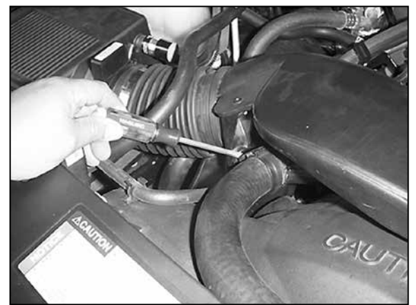
5. Using a flat blade screwdriver, pry the radiator hose retaining clip from the intake tube.
