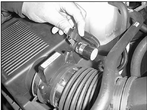
2. Disconnect the mass air sensor electrical connection.
