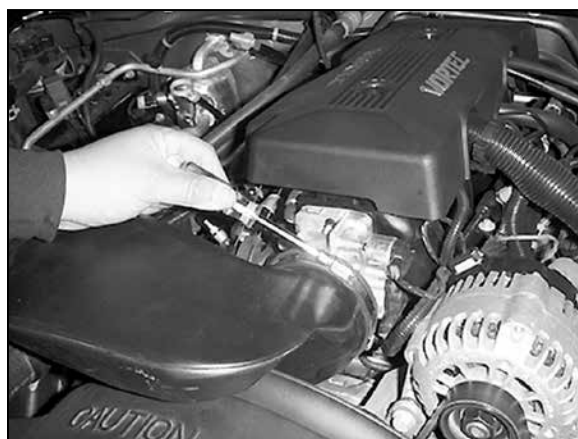
4. Loosen the hose clamp on the intake tube at the throttle body.
