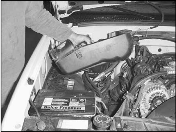
8. Remove the lower airbox assembly. NOTE: K&N Engineering, Inc., recommends that customers do not discard factory air intake.
