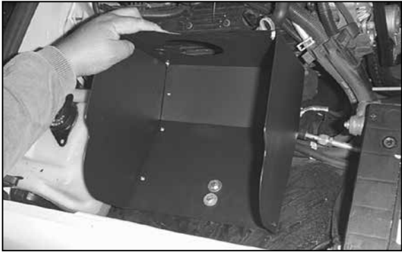
23. Install the heat shield assembly into the two holes on the inner fender and secure from underneath. NOTE: Apply the poron gasket onto the heatshield to cover the exposed bolts.
