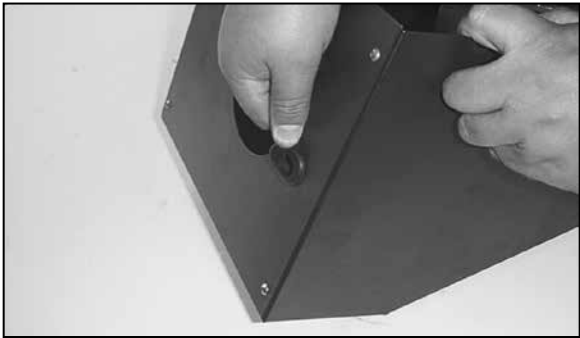
19. Install the provided grommet into the small hole on the heat shield.
