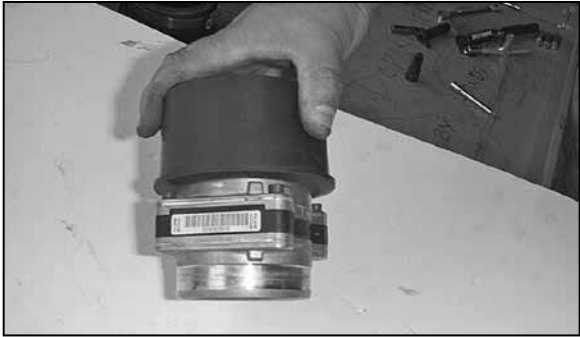
21. Install the filter adapter onto the mass air sensor with the directional arrow as shown above.
