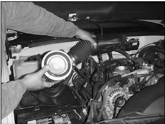
7. Lift and remove the complete air intake system.
