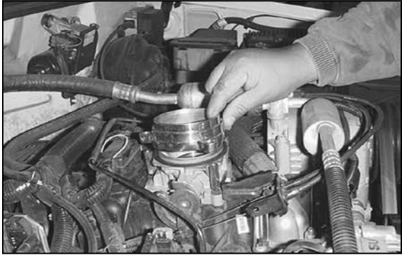
16. Install the aluminum throttle body adapter and hand start the three 6mm allen bolts.
