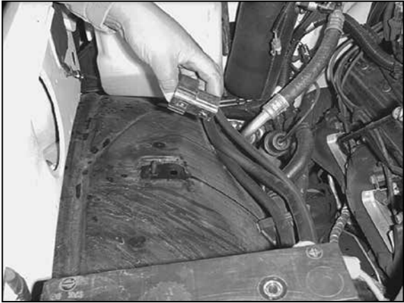
9. Using a 13mm socket, remove lower airbox bracket from inner fender.
