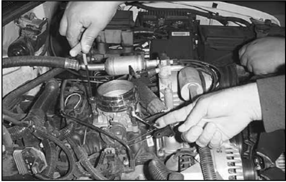
17. Using a 7/16" wrench, snug the three coupling nuts and tighten the three 6mm bolts using a 5mm allen wrench.
