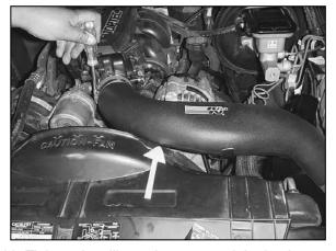
22. Tighten the silicone hose around the intake tube with the hose clamp provided.
