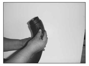
19. Remove the air temperature sensor from the factory intake hose and reinstall it into the grommet hole on the underside of the K&N® intake tube as shown above.
