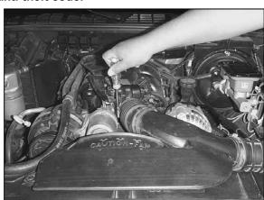
2. Loosen the hose clamp located on the rubber intake hose at the throttle body.
