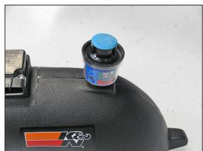
11. Install the factory grommet and filter restriction gauge into the  $K\&N^{\scriptsize @}$  intake tube as shown.
