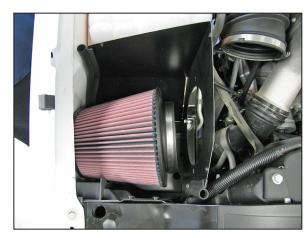
17. Set the K&N® filter into the heat shield as shown.
