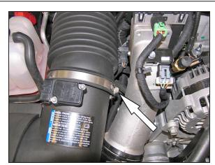
3. Loosen the hose clamps which secure the air filter housing to the stock intake tube.
