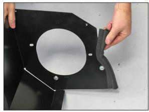
15. Install the edge trim onto the heat shiels as shown
