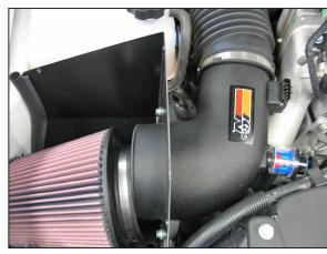
18. Install the K&N® intake tube into the heat shield and into the stock intake tube, then secure the K&N® intake tube to the heat shield with the hardware provided and hose clamp at the stock intake tube.
