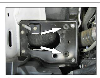
5. Remove the two mounting grommets shown from the mounting plate.
