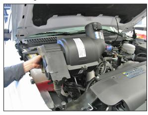
4. Lift up the air filter housing to release it form the mounting grommets, and then remove the air filter housing from the vehicle as shown.
