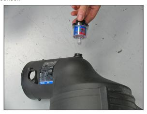
8. Remove the air filter restriction gauge and stock grommet from the air filter housing as shown.
