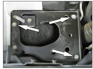
6. Remove the three bolts shown which secure the mounting plate.
