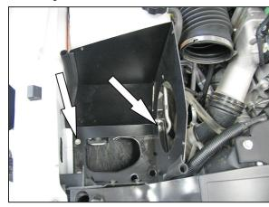
16. Install the heat shield onto the air box mounting plate and secure with the factory bolts removed in step #6.
