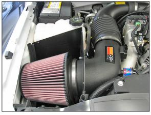
19. Install the K&N $^{\circ}$  filter onto the K&N $^{\circ}$  intake tube and secure with the provided hose clamp.
