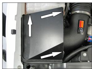
21. Install the heat shield lid onto the heat shield and secure with the three 5mm button head allen bolts provided.
