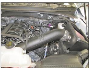
Install the K&N<sup>®</sup> intake into the coupling hose at the filter adapter and then into the hose at the throttle body, adjust the tube for best fit and then secure with the provided hose clamps.
