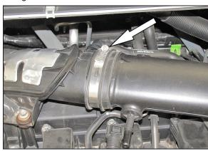
4. Loosen the hose clamp that secures the intake tube to the turbo inlet.
