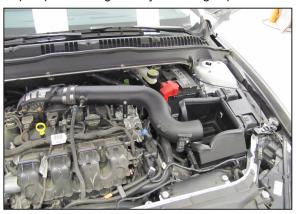
17. Install K&N® intake tube into the hose and onto the tube mounting bracket. Align with heat shield and secure with provided hardware.
