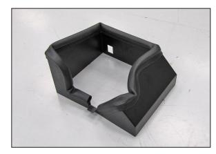
15. Install edge trim onto heat shield as shown. **NOTE: Some trimming of the edge trim will be necessary.**
