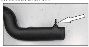
14. Install provided  $\frac{1}{4}$  NPT quick connect fitting onto the K&N® intake tube.
