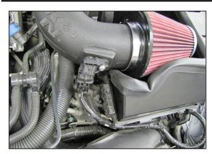
20. Reconnect pressure sensor electrical connector onto sensor.
