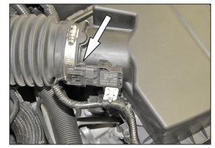
6. Disconnect the temperature sensor electrical connect.
