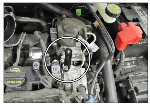
10. Attach tube bracket 07158 onto engine with provided hardware. Do not completely tighten at this time.
