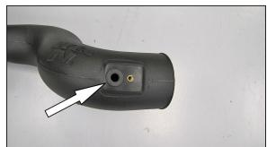
12. Install provided grommet into K&N<sup>®</sup> intake tube
