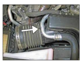
7. Unhook the coolant pipe from the intake tube.
