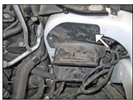
17. Remove the push pin securing the top of the fresh air intake duct.
