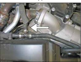
8. Loosen the hose clamp that secures the intake tube to the engine inlet.
