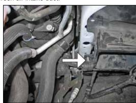
18. Unhook the wiring harness secured to the core support through the fresh air intake duct.
