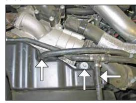
6. Unhook the coolant hoses from the intake plenum and remove the bolt securing the plenum to the engine fan shroud.
