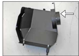
21. Install the filter adapter into the heat shield using the provided hardware.
