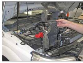
19. Remove the fresh air intake duct from the vehicle. Secure the inner fender to the vehicle with the original hardware from step #15.
