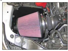
38. Feed the K&N® air filter top first into its location, then rotate it back and install onto the filter adapter. Secure the air filter with the provided hose clamp.
