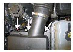
5. Release the three retaining clips that secure the upper air box to the lower air box.
