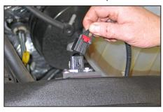
24. Connect the provided mass air sensor extension harness into the factory harness connection, and then connect the open end to the mass air senor electrical connector.
