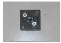
19. Install the mass air sensor into the mass air adapter and secure with the provided screws.
