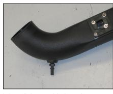
21. Install the provided crank case vent fitting into the  $K\&N^{\text{\$}}$  intake tube as shown.
