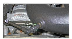
23. Rotate the crank case vent coupler so that it lines up with the fitting installed in the K&N<sup>®</sup> intake tube, then connect the coupler to the fitting.
