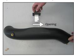
20. Install the mass air sensor assembly into the  $K\&N^{\otimes}$  intake tube as shown.
