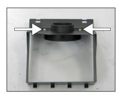
9. Install the K&N® filter adapter into the heat shield as shown and secure with the provided hardware.
