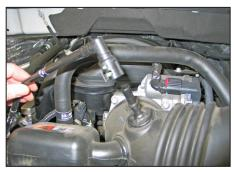
3. Release the green locking tab and then disconnect the crank case vent line from the intake tube as shown.
