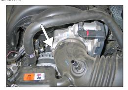
4. Loosen the hose clamp which secures the intake tube to the throttle body.
