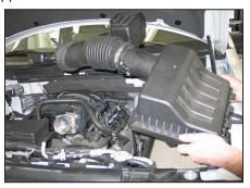
6. Remove the upper air box housing and intake tube assembly from the vehicle.
