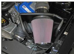
24. Install the  $K\&N^{\otimes}$  air filter and secure with the provided hose clamp.
