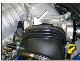
6. Loosen the hose clamp securing the stock intake tube to the throttle body.
