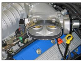
19. Install the provided silicone hose (08627) onto the throttle body and secure with the provided hose clamp.
