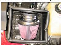
23. Place the air filter assembly into the heat shield as shown.
