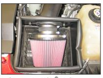
25. Secure the K&N<sup>®</sup> air filter assembly onto the K&N<sup>®</sup> intake tube with the provided hose clamp as shown.
