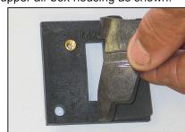
11. Install the provided gasket onto the mass air adapter as shown with the sticky side down.
