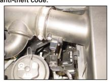
2. Release the red locking tab and disconnect the mass air sensor electrical connection.
