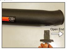
13. Install the mass air sensor assembly into the intake tube.
