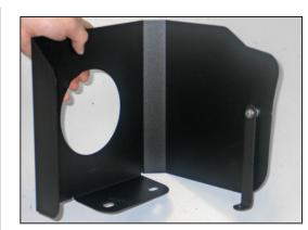
6. Install "L" bracket (#070026) onto the heat shield with the provided hardware.
