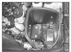
10. Install the heat shield and secure with the provided hardware as shown. **NOTE:** Due to vehicle manufacturing inconsistencies, some vehicles may not be equipped with the threaded hole in the factory filter mounting plate. In this case, it will be necessary to drill a 1/8" ID hole in the filter mounting plate and attach the heat shield mounting bracket with the provided sheet metal screw.
