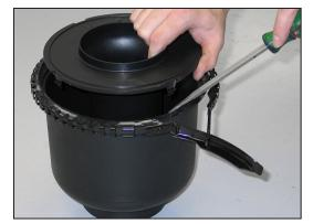
14. Using a flat blade screw driver; push in and release the four clips that secure the mass air sensor retaining plate.
