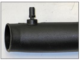
19. Install the  $1\!\!\!/4"$  NPT fitting into the K&N® intake tube as shown.
