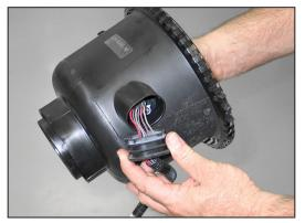
12. Slide the rubber wiring harness plug back, exposing the mass air sensor electrical connection.
