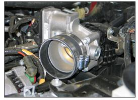
20. Install silicone hose (#08690) onto the throttle body and secure with the provided hose clamp.
