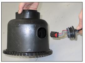
13. Release the mass air sensor electrical connection.
