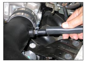
24. Connect the provided crank case vent hose onto the fitting on the valve cover and the vent fitting on the  $K\&N^{\otimes}$  intake tube.
