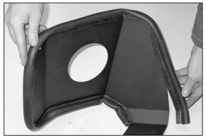
17. Install the supplied edge trim onto the heat shield as shown.
