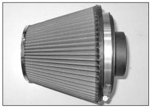
31. Install the filter adapter into the K&N<sup>®</sup> air filter as shown and secure with the provided hose clamp.
