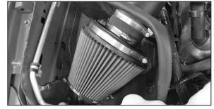
33. Install the air filter assembly onto the K&N intake tube and secure with the provided hose clamp.
