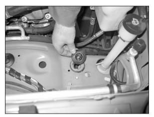
12. Remove the front lower air box mounting grommet shown.
