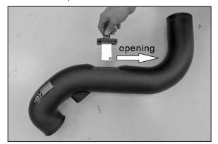
26. Install the mass air sensor assembly into the K&N $^{\circ}$  intake tube and secure with the provided hardware.
