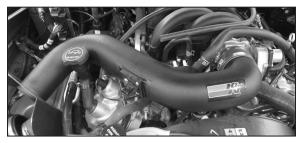
28. Install the K&N<sup>®</sup> intake tube into the silicone hose at the throttle body and align with the mounting bracket installed in step #16. Secure the intake tube with the hose clamp and supplied hardware.
