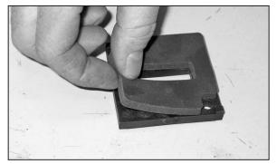
24. Install the supplied gasket onto the mass air sensor adapter as shown.
