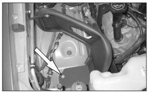
NOTE: The lower air box housing is attached to the inner fender well at four locations. NOTE: K&N Engineering, Inc., recommends that customers do not discard factory air intake.
