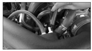
30. Install the supplied brake booster vent hose onto the factory fitting and then connect the other end to the npt fitting in the K&N<sup>®</sup> intake tube.
