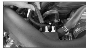
29. Install the supplied shorter crank case vent line onto the fitting on the valve cover and then onto the npt fitting installed in the K&N<sup>®</sup> intake tube.
