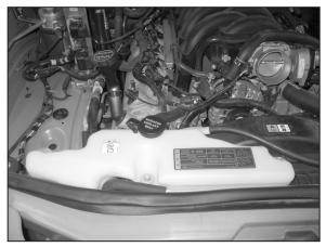
11. Reinstall the coolant recovery tank and secure with the factory bolts removed in step #8.
