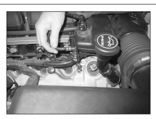
3. Rotate the green locking ring clockwise, then unhook the crank case vent hose from the valve
