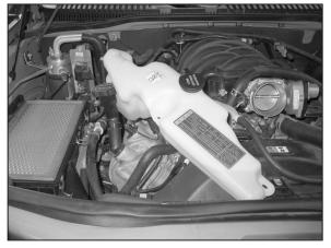
9. Lift and position the coolant recovery tank on the engine to gain access to the lower air box. Note: Use care when moving the coolant recovery tank as the recovery hose will still be attached to the radiator.
