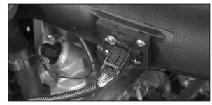
34. Reconnect the mass air sensor electrical connection.
