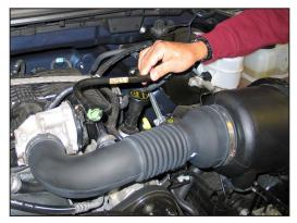
2. Rotate the crank case vent hose locking rings and pull the crank case vent hose off of the valve cover and intake tube as shown. 3. Loosen the hose clamps that secure the stock intake tube to the throttle body and air filter housing; remove the intake tube from the vehicle.
