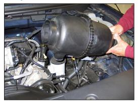
4. Firmly pull up the assembly to unhook it from the mounting grommets and inner fender as shown. NOTE: Use caution as the mass air sensor electrical harness will still be connected. NOTE: K&N Engineering, Inc., recommends that customers do not discard factory air intake. 5. Unhook the secondary mass air sensor connection from the clip that secures it to the
