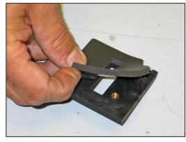
19. Install the supplied gasket onto the mass air sensor adapter as shown.
