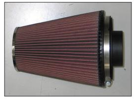
24. Install the filter adapter into the K&N<sup>®</sup> air filter and secure with the provided hose clamp.
