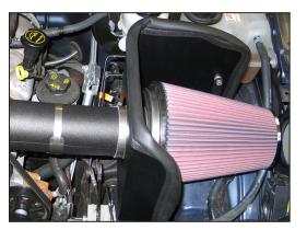
26. Install the filter assembly onto the intake tube and secure with the provided hose clamp. NOTE: Drycharger<sup>®</sup> air filter wrap; part # RC-5046DK is available to purchase separately. To learn more about Drycharger<sup>®</sup> filter wraps or look up color availability please visit http://www.knfilters.com<sup>®</sup>.
