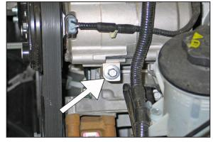
8. Remove the lower front A/C compressor mounting bolt shown. **NOTE: This bolt will be reused.**
