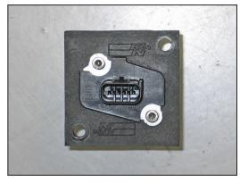
20. Install the mass air sensor into the adapter using the provided bolts.
