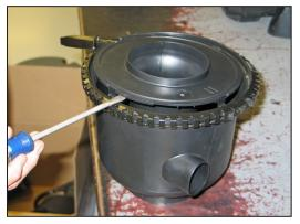
17. Using a flat blade screwdriver, push in and release the mass air retaining plate clips and lift as shown.
