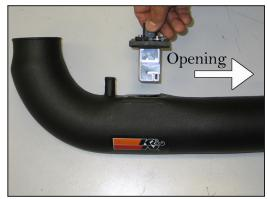
21. Install the mass air sensor assembly into the  $K\&N^{\textcircled{o}}$  intake tube and secure with the provided hardware.
