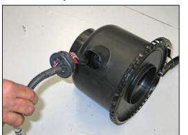
16. Slide the rubber grommet back to gain access to the mass air sensor electrical connector. Using a
