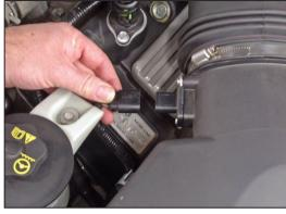
2. Depress the locking tab and then unhook the mass air sensor electrical connection.
