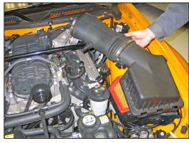
7. Remove the intake tube and airbox lid from the vehicle.
