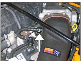
26. Attach the crankcase vent hose to the factory fitting that was installed in the K&N® intake tube in step #15.
