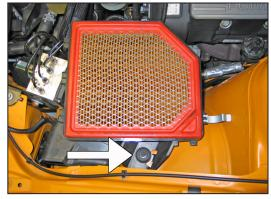
8. Remove the lower airbox retaining bolt shown.
