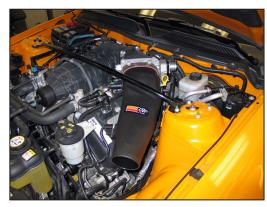
20. Install the K&N® intake tube into the throttle body and align with the mounting bracket, then secure with the provided hose clamp and hardware.
