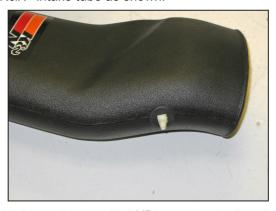
13. Insert the supplied  $\frac{1}{4}$ " hose mender into the grommet that was installed in the previous step.
