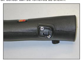
11. Install the mass air sensor into the  $K\&N^{\otimes}$  intake tube and secure with the provided spacers and m4 bolts.
