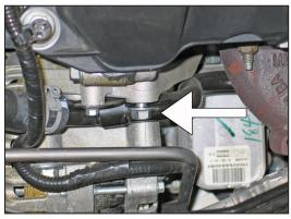
18. Remove the upper alternator mounting bolt shown
