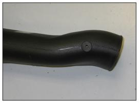
12. Install the supplied  $\frac{1}{4}$ "id vent grommet into the K&N® intake tube as shown.
