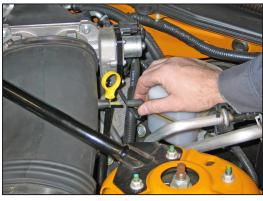
4. Disconnect the vacuum vent line as shown.
