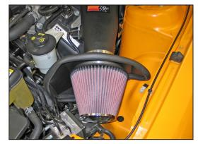
24. Set the filter assembly into the position. Slide the silicone hose onto the filter adapter's inlet and and secure the filter assembly to the intake tube with the provided hose clamps.
