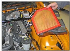
9. Remove the lower airbox housing from the vehicle.
