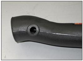
14. Install the supplied crankcase vent grommet into the  $K\&N^{\otimes}$  intake tube as shown.
