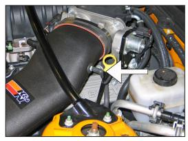
25. Connect the vacuum vent line onto the ½" hose mender that was inserted in the K&N® intake tube during step #13.
