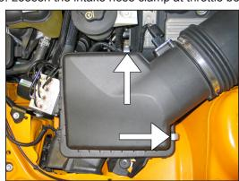
6. Unlatch the two upper airbox retaining clips shown.
