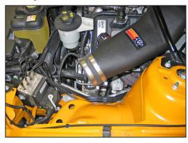
23. Install the silicone hose (08761) onto the intake tube and slide it past the bead on the end of the tube so proper clearance is maintained when the air filter assembly is installed.
