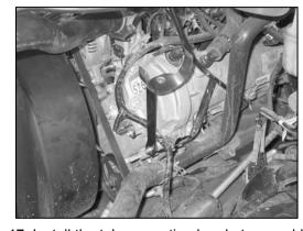
17. Install the tube mounting bracket assembly onto the threaded stud with the spacer installed in step #15. Then secure with the provided hardware.
