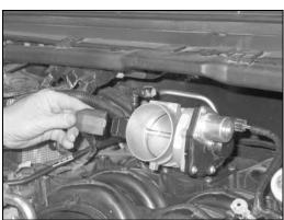
14. Reconnect the throttle body motor and TPS sensor electrical connections.
