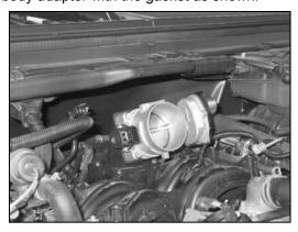
13. Install the throttle body assembly onto the intake manifold with the provided hardware as shown.
