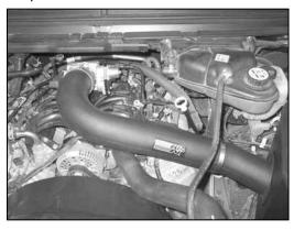
32. Install the K&N® intake tube into the silicone hose at the throttle body and onto the saddle clamp, then secure with the provided hose clamps.
