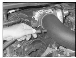
34. Install the supplied crank case vent hose onto the valve cover fitting and then onto the K&N® intake tube as shown.
