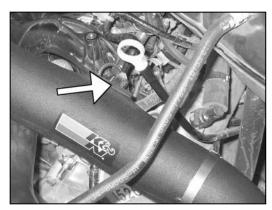
38. Install the filter adapter assembly into the K&N® filter and secure with the provided hose clamp.
