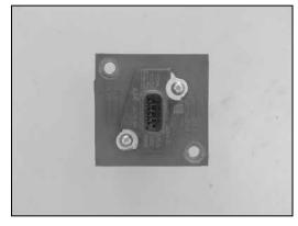
28. Install the mass air sensor into the K&N® adapter and secure with the provided hardware.
