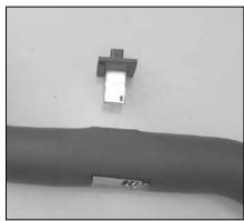
29. Install the mass air sensor assembly into the  $K\&N^{\otimes}$  intake tube.
