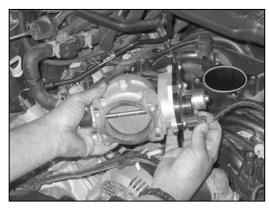
11. Lift the throttle body from the intake manifold. Then disconnect the throttle body motor electrical connection.
