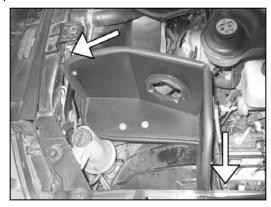
25. Secure the heat shield mounting brackets with the factory bolts removed in step #20 and #21. Tighten the mounting brackets to the heat shield.
