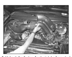
5. Unhook the factory fresh air tube from stock air box and radiator core support. Then remove the fresh air tube from the vehicle.
