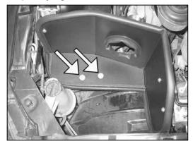
24. Place the heat shield onto the fender well so that it will align onto the lower bracket. Secure the heat shield to the lower bracket with the hardware provided as shown.
