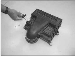
26. Remove the two screws securing the mass air sensor to the factory air box. Then remove the sensor from the air box.
