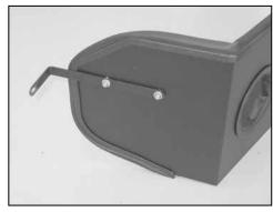
22. Install the large "L" bracket (010060) onto the heat shield as shown with the provided hardware. NOTE: Be sure to place a flat washer between the heat shield and bracket as a spacer. Do not completely tighten at this time.
