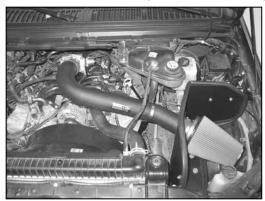
39. Install the filter adapter assembly into the K&N® filter and secure with the provided hose clamp.
