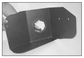
18. Install the short edge trim into the hole in the heat shield as shown.
