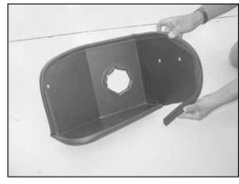
19. Install the long edge trim around the heat shield as shown.
