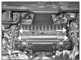
6. Remove the four air filter housing bolts shown.
