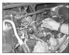
33. Remove the factory crank case vent hose from the valve cover.
