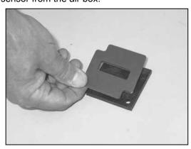
27. Install the provided gasket onto the K&N $^{\! \otimes}$  mass air sensor adapter as shown.
