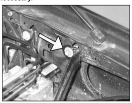
20. Remove the anti lock brake mounting bolt shown.
