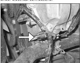
15. Install the provided spacer onto the threaded stud in the cylinder head.
