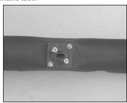
30. Secure the mass air sensor assembly to the K&N® intake tube with the provided hardware.
