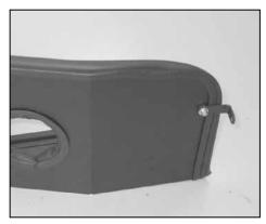
23. Install the small "L" bracket (010060) onto the heat shield as shown with the provided hardware. NOTE: Be sure to place a flat washer betweeen the heat shield and bracket as a spacer. Do not completely tighten at this time.
