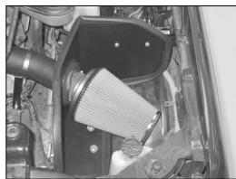
37. Install the filter adapter assembly into the K&N® filter and secure with the provided hose clamp.
