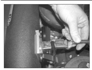
37. Reconnect the mass air sensor electrical connection.
