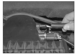
4. Disconnect the brake booster vent line from the air filter housing as shown.
