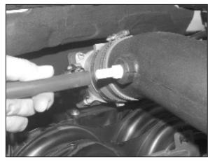
33. Install the provided silicone vent hose onto the valve cover and onto the  $K\&N^{\scriptsize \$}$  intake tube as shown
