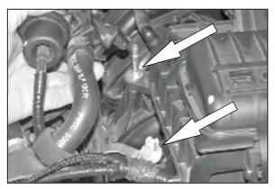
5. Pull up on the heater control valve and wiring harness mounting clips to unhook them from the air box mounting studs as shown.
