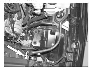
13. Loosen the coolant recovery hose, hose clamps, and then remove the factory recovery hose shown. Be sure to catch any coolant, which flows out of the radiator during hose removal.
