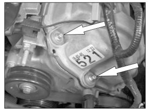
27. Remove the two valve cover mounting bolts shown.
