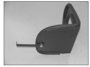
17. Install the "L" bracket (#070026) onto the heat shield with the provided spacer and hardware as shown
