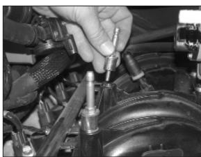
35. Re-install the factory air box mounting studs with the provided spacers as shown.
