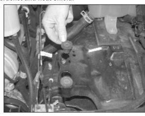
18. Install the provided nut inserts into the air box mounting holes as shown.
