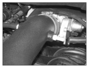
34. Install the factory brake booster vent hose to the K&N® intake tube as shown.
