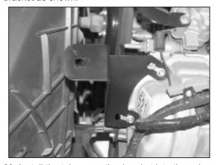
29. Install the tube mounting bracket into the valve cover using the factory bolts. Do not completely tighten the bolts at this time
