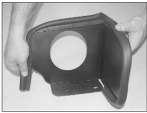
15. Install the long edge trim onto the heat shield as shown.
