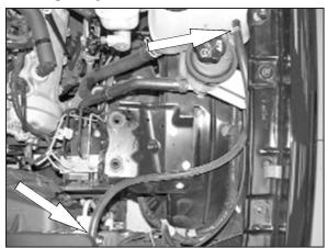
14. Install the supplied coolant recovery hose and secure with the provided hose clamps.
