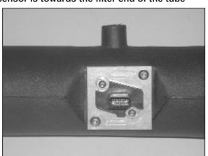
25. Secure the mass air sensor assembly onto the K&N® intake tube with the provided hardware as shown.
