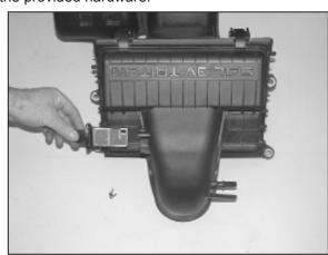
21. Remove the two screws that secure the mass air sensor to the air box with the wrench provided. Then remove the mass air sensor.
