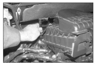
3. Rotate the crank case vent hose locking ring and pull the crank case vent hose off of air filter housing. Unhook the wiring harness retaining clip from the air box.
