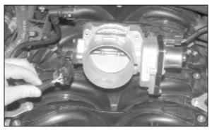
12. Reconnect the throttle body motor and TPS electrical connections.
