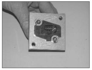
23. Install the mass air sensor into the K&N® mass air adapter as shown and secure with the provided hardware.
