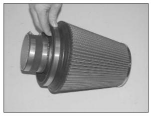
39. Install the adapter assembly into the K&N® air filter as shown. Tighten hose clamp.
