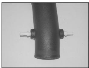
26. Install the provided NPT fittings into the intake tube as shown.
