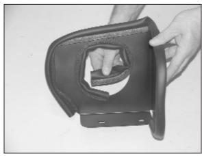
16. Install the short edge trim into the hole in the heat shield as shown.
