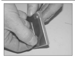
22. Install the provided gasket onto the K&N $^{\!0}$  mass air adapter as shown. Sticky side down.
