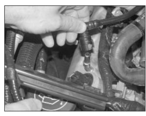
32. Unlock the crank case vent hose and remove the hose from the valve cover.
