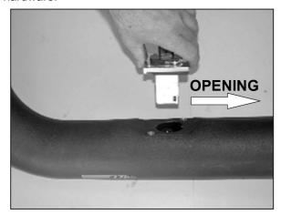
24. Install the mass air sensor assembly into the K&N® intake tube.
