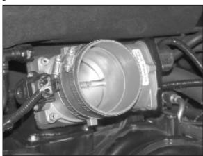
30. Install silicone hose (#08630) onto the throttle body with the provided hose clamps as shown.
