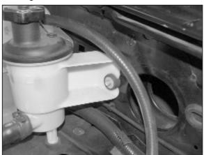
19. Remove the power steering reservoir mounting bolt shown.
