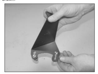
28. Pass the two valve cover bolts, removed in step #27, through the keyhole slots in the tube mounting bracket as shown.
