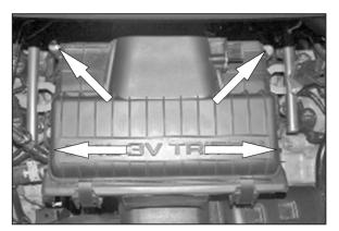
6. Remove the four air box mounting bolts shown, with a 10mm socket.
