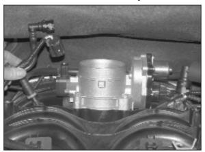
8. Disconnect the TPS sensor electrical connection from the throttle body. Then remove the four throttle body mounting bolts.
