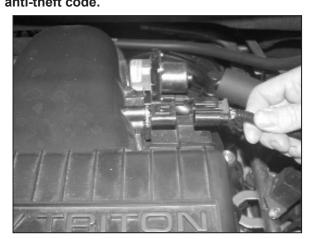
2. Disconnect mass air sensor electrical connection.
