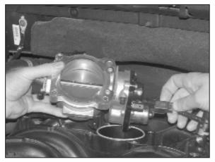
9. Lift the throttle body from the intake manifold. Then disconnect the throttle body motor electrical connection.
