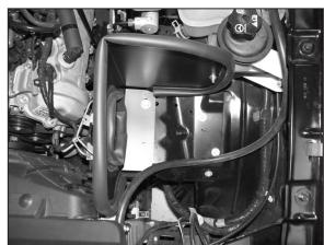
20. Install the heatshield as shown and secure with the provided hardware.
