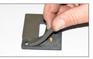
12. Peel the backing paper from the mass air sensor adapter plate gasket and install the gasket onto the mass air sensor adapter plate sticky side down.
