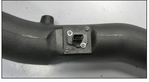
15. Secure the mass air sensor assembly into the  $K\&N^{\otimes}$  intake tube with the provided hardware.
