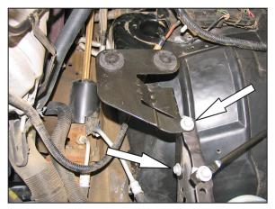
7. Remove the two bolts, which secure the air box mounting bracket shown, and then remove the airbox mounting bracket.
