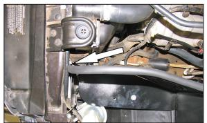
10. Remove the upper air box mounting bracket bolt shown.
