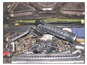
4. Loosen the hose clamps, which secure the intake tube to the throttle body and to the air box, then remove the intake tube from the vehicle.
