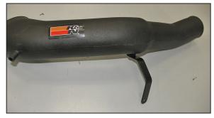
25. Install the tube mounting bracket (26624) onto the K&N<sup>®</sup> intake tube and secure with the provided hardware as shown.
