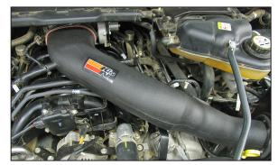
26. Install the K&N<sup>®</sup> intake tube onto the throttle body and align the mounting bracket so that it sits on the 8mm stud protruding from the cylinder head.
