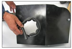
18. Install the edge trim into the heat shield opening as shown.
