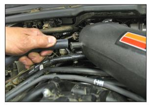
29. Install the crank case vent hose onto the K&N $^{\mbox{\tiny \$}}$  intake tube as shown.
