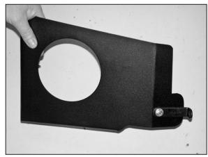
10. Install the "L" bracket (07158) onto the front of the heat shield as shown with the provided
