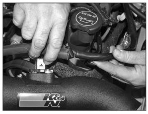
19. Install the provided crankcase vent hose onto the K&N $^{\circ}$  intake tube and factory vent hose as shown.
