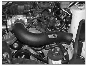
17. Install the K&N<sup>®</sup> intake tube into the silicone hose at the throttle body and onto the tube-mounting bracket installed in step #8, secure with provided hardware.
