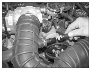
3. Release the locking ring and then disconnect the crank case vent tube.
