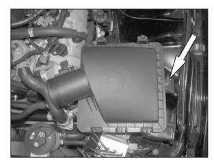
5. Remove the airbox mounting bolt shown.
