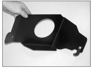
9. Install the "L" bracket (070812) onto the rear of the heat shield as shown with the provided hardware.
