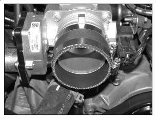
16. Install the silicone hose (08434) onto the throttle body with the provided hose clamps as shown.
