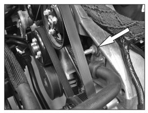
7. Remove the power steering pump bracketretaining nut shown. **NOTE: Nut will be reused.**
