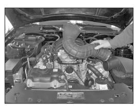
4. Loosen the hose clamps, which secure the intake tube to the throttle body and air box, then remove the intake tube as shown.
