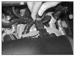
26. Reconnect the mass air sensor electrical connection as shown.
