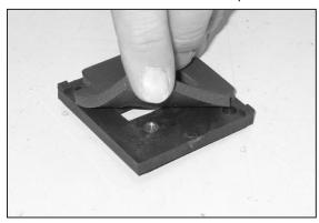
17. Install the provided gasket to the back of the  $K\&N^{\tiny \circledcirc}$  mass air sensor adaptor plate as shown.
