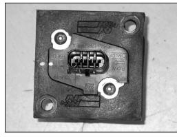
17a. Install the mass air sensor into the K&N® mass air sensor adaptor and secure with the provided hardware.
