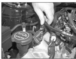
3. Rotate the green locking tab clockwise and then disconnect the crank case breather hose from the valve cover as shown.
