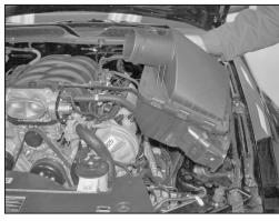
6. Remove the air box assembly as shown.
