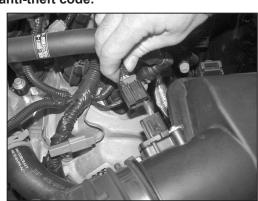
2. Release the red locking tab and then disconnect the mass air sensor electrical connection.
