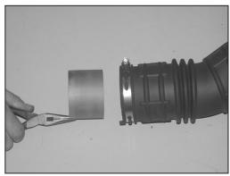
21. Vehicles that come equipped with Hydrocarbon trap, use a pair of needle nose pliers, to remove the Hydrocarbon trap from the stock intake tube as shown.
