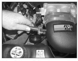
20. Install the supplied vent hose onto the vent port on the valve cover and then onto the  $K\&N^{\otimes}$  intake tube as shown.
