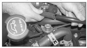
16. Cut the factory crank case vent tube one inch from the end, then attach the supplied silicone vent hose to the K&N<sup>®</sup> intake tube and factory vent tube as shown.
