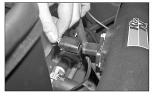
20. Reconnect the mass air sensor electrical connection.
