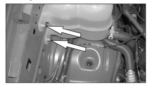
10. Remove the two-coolant bottle mounting bolts and the forward air box retaining grommet shown.
