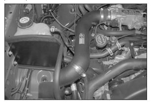
15. Install the K&N<sup>®</sup> intake into the silicone hose at the throttle body and onto the saddle clamp, then secure with the provided hose clamp.
