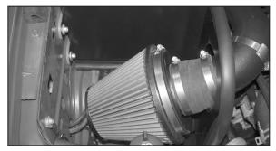
19. Install the filtercharger assembly onto the  $K\&N^{\ensuremath{\circledast}}$  intake tube and secure with the provided hose clamp as shown.
