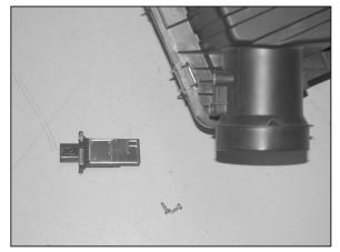
6. Using the "TORX" L key provided, remove the two screws, which retain the mass air sensor to the air box then remove the sensor as shown.
