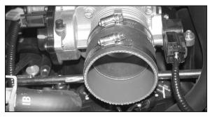
13. Install the silicone hose (08192) onto the throttle body and secure with the provided hose clamp as shown.
