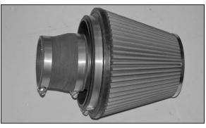
18. Install the silicone hose (08724) onto the filtercharger assembly and secure with the provided hose clamp as shown.
