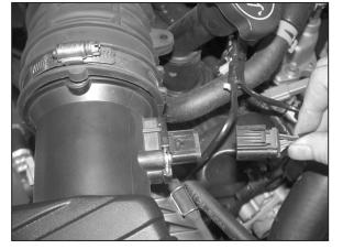
2. Depress the red locking tab and then disconnect the mass air sensor electrical connection.
