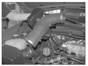
4. Loosen the hose clamps at the throttle body and the air box, and then remove the stock intake tube as shown.
