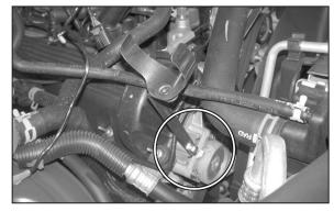
8. Using the 8mm bolt washers supplied, attach the tube mounting bracket assembly to the front of the engine at the threaded boss above the belt tensioner as shown.
