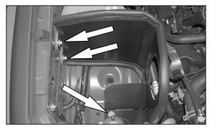
12. Install the heat shield as shown and attach to the inner fender with the factory coolant bottle mounting bolts and the 3/8" bolt and washer provided.
