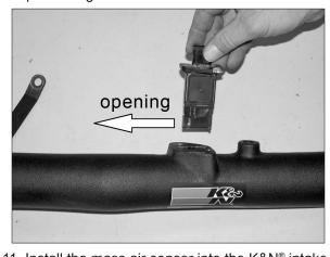
11. Install the mass air sensor into the K&N® intake tube with the open end of the sensor pointed towards the filter end of the tube.
