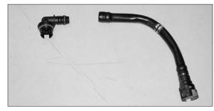
25. Using a razor blade slit the plastic tube and then remove the tube from the valve cover fitting as shown.
