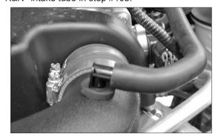
16b. On vehicles equipped with a brake booster breather line, connect the vent line to the 90° fitting installed in step #16a.
