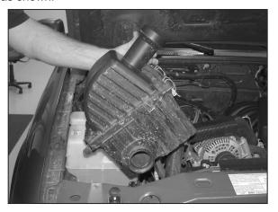
6. Slide a flat blade screwdriver in between the airbox and the airbox mounting tray. Pry downward on the tray, while pulling upwards on the airbox assembly to release the assembly from the retaining grommets in the tray.
