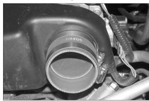
15. Install the provided silicone hose (08405) onto the throttle body as shown.
