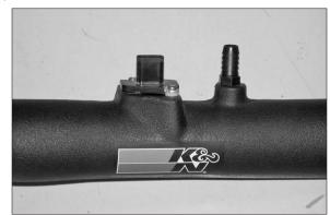
13. Install the vent fitting into the new intake tube
