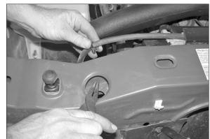
17. Using small pliers, squeeze the cooling system reservoir hose-retaining clip through the large hole in the top of the core support, and then remove the clip from the radiator core support.
