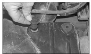
21. Install the threaded inserts to the airbox mounting bracket as shown.
