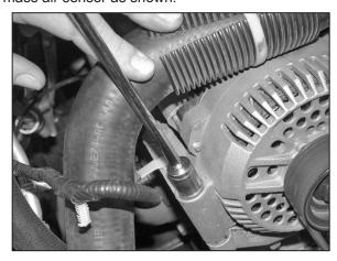
9. Loosen and remove the lower front alternator hex bolt as shown.
