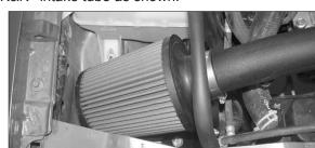
28. Install the K&N® air filter onto the intake tube and secure with the provided hose clamp as shown.
