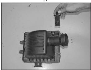
8. Remove the two mass air retaining screws with the torx wrench provided, and then remove the mass air sensor as shown.
