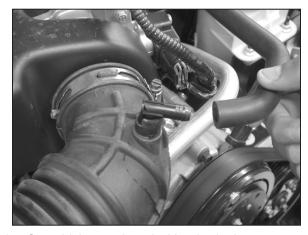
3a. On vehicles equipped with a brake booster breather line, disconnect the breather line from the factory 90° fitting as shown.
