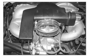
21. Install the silicone hose (08623) onto throttle body with provided hose clamps as shown.
