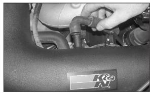
25. Install the air temp sensor into the K&N® intake tube, reconnect the air temp electrical connection and install crank case vent onto the vent port.
