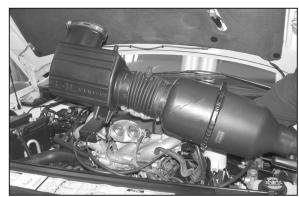
8. Remove the entire stock intake assembly. NOTE: K&N Engineering, Inc., recommends that customers do not discard factory air intake.
