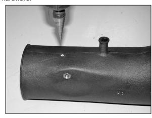
19. On vehicles equipped with an air temp sensor. Drill a 5/8" hole at the drill point indicated on the K&N® intake tube.
