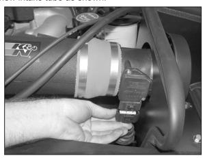
29. Reconnect the primary and secondary mass air electrical connection.
