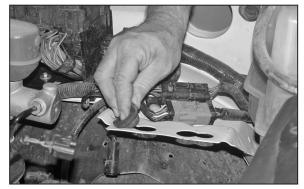
13. Remove the two air box mounting grommets from vehicle as shown.
