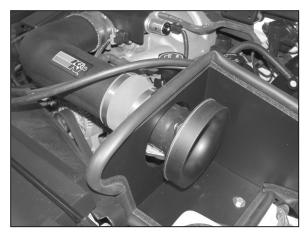
28. Install the mass air sensor assembly onto the new intake tube as shown.
