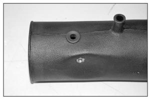
20. Install the provided grommet into the new intake tube as shown.
