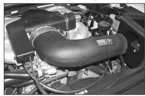
23. Install the new K&N® intake tube onto the silicone hose.
