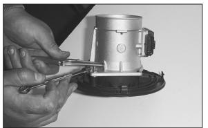
12. Using a pair of small vise grips or pliers, hold the stud while using a 10mm wrench to loosen the nuts, then remove the mass air sensor from the retaining plate.
