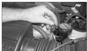
3. On vehicles equipped with air temp sensor, disconnect wire connector from air temp sensor.
