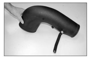
22. Install the provided bracket (07169) onto the K&N® intake tube with hardware provided.
