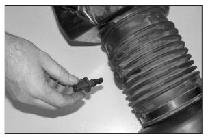
24. On vehicles equipped with air temp sensor, remove the air temp sensor from the stock intake tube.
