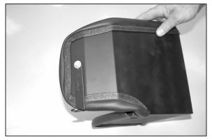
16. Install the provided "L" bracket (070952) onto heat shield as shown.
