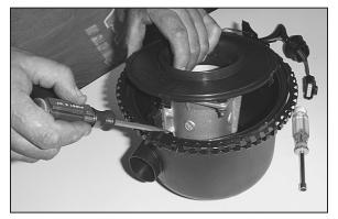
12. Using a flat blade screwdriver, push in and release the four clips that retain the mass air sensor retaining plate.
