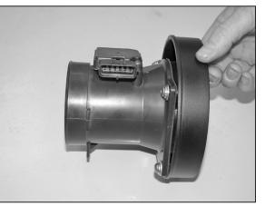
14. Attach the mass air adapter to the mass air sensor using the gasket and hardware provided as shown.
