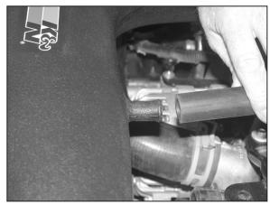
19. Install the provided silicone vent hose onto the valve cover and onto the K&N $^{\circ}$  intake tube as shown.
