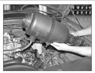
5. Pull firmly up on the air filter assembly to remove it from the mounting grommets.
