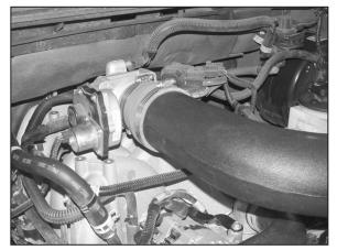
17. Install the K&N<sup>®</sup> intake tube into the silicone hose on the throttle body and secure with the provided hose clamp.
