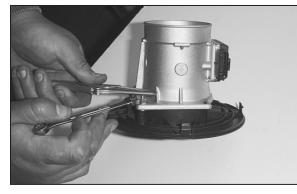
13. Using a pair of small vise grips or pliers, hold the stud while using a 10mm wrench to loosen the nuts, then remove the mass air sensor from the retaining plate.
