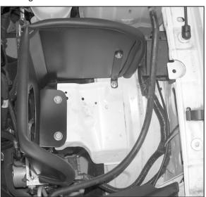
9. Install the heatshield as shown and secure with the provided hardware.
