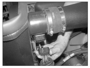
22. Reconnect the primary and secondary mass air sensor electrical connections.
