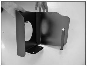
6. Install "L" bracket (070026) onto the heatshield with the hardware provided as shown.
