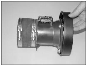
20. Install the provided silicone hose (08626) onto the mass air assembly and secure with the provided hose clamp.
