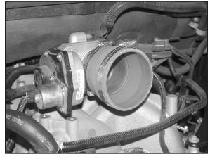
15. Install silicone hose (08724) onto the throttle body with the provided hose clamp as shown.
