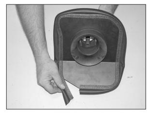
15. Install the edge trim onto the heat shield as shown. Trim if needed.
