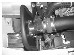
17. Install the mass air assembly onto the intake tube then secure with the provided hose clamps.
