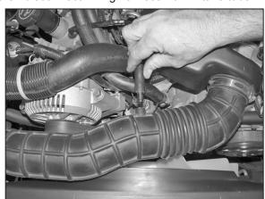
3. Disconnect the crank case vent from intake tube as shown.
