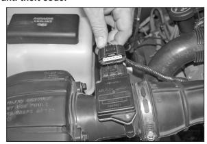
2. Disconnect the mass air elcetrical connection, then disconnect wiring harness from intake tube.
