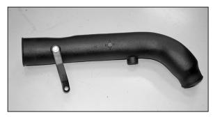
10. Mount the provided bracket onto the new K&N® intake tube with the provided hardware as shown.
