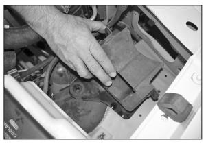
7. Pull firmly on the air inlet duct to release the duct from the radiator core support as shown.
