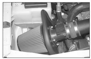
19. Install the K&N® filtercharger onto the mass air assembly as shown.
