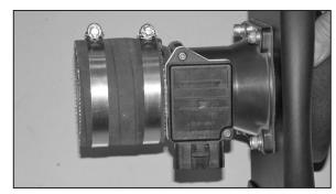
16. Install the silicone hose (08192) onto the throttle body usign the provided hose clamps.
