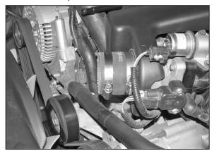
12. Install the provided silicone hose (08405) onto the throttle body as shown.
