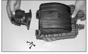
8. Loosen and remove the four hex bolts that secure the mass air sensor, then, remove the mass air sensor from the air cleaner as shown.
