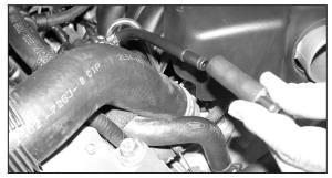
5. Remove rubber hose from crank case vent line as shown.
