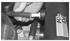
18. Install the provided siliocne hose onto the crank case vent line, then attach to the intake tube as shown.
