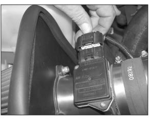
20. Reconnect the mass air electrical connection as shown.
