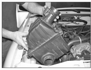
6. Slide a flat blade screwdriver in between the air cleaner and the air cleaner mounting tray. Pry downwards on the tray, while pulling upwards on the air cleaner assembly to release the assembly from the retaining grommets in the tray.
