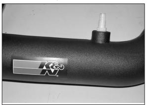
11. Install the vent fitting into the new intake tube
