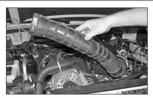
4. Loosen the hose clamps at the throttle body and at the mass air sensor, then remove the intake tube as shown.
