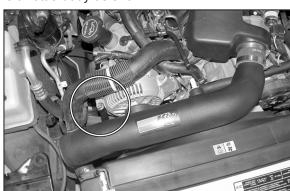
13. Install the intake tube onto the throttle body, then using the bolt removed in step #9 secure the bracket onto the alternator as shown.
