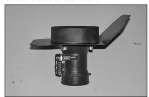
14. Assemble the mass air adaptor, heat shield, gaskets and the mass air sensor as shown using the provided hardware.
