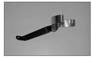
18a. On vehicles that come equipt with A/C, assemble the saddle bracket assembly as shown using bracket (07181).
