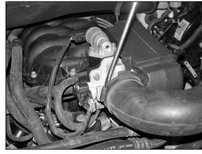
4. Loosen hose clamp at the throttle body.
