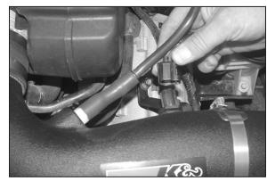
28. Reconnect the temp sensor electrical connection as shown.
