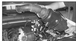
7. Remove the entire stock air intake assembly from the vehicle.
