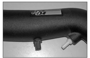
23. Install the temp sensor into the new K&N® intake tube as shown.
