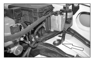
14. Remove the 6mm bolt that retains the cruise control onto vehicle.
