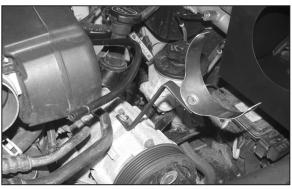
19. On vehicles that come equipt with A/C, remove the A/C mounting bolt. Then secure saddle bracket assembly from step 18a onto vehicle with the bolt that was removed.
