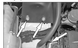
17. On vehicles with cruise control install heat shield as shown with the provided hardware.
