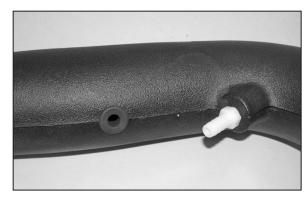
22. Install the provided grommet and vent fitting onto the new K&N® intake tube as shown. **NOTE: Plastic NPT fittings are easy to cross** thread. Install the vent fitting "hand" tight, then turn it two complete turns with a wrench.
