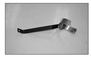
18. On vehicles that did not come equipt with A/C, assemble the saddle bracket assembly as shown using bracket (07180).
