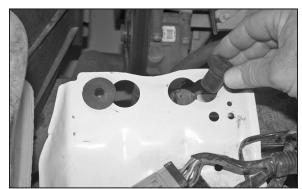
16. Install the two nut inserts onto the air box mounting tray as shown.
