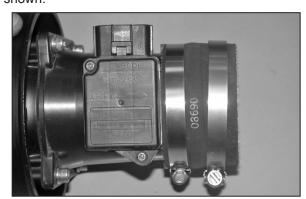
25. Install the silicone hose (08690) onto the mass air assembly with the provided hose clamps as shown.
