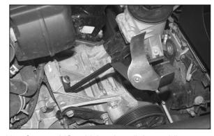
19a. On non A/C vehicles, install the saddle bracket assembly from step 18 onto vehicle with the provided hardware as shown.
