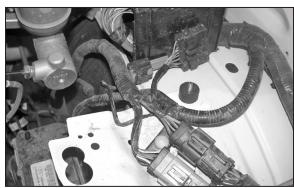
14a. On vehicles without cruise control, install the rubber mounted stud onto vehicle as shown.
