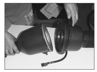
8. Open the air cleaner assembly and isolate the mass air sensor assembly.
