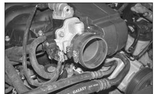
20. Install the provided silicone hose (08756) onto the throttle body with the provided hose clamps.
