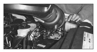
5. Detach the stock intake tube from the throttle body and lift up on the air cleaner assembly to release it from it's retaining grommets.
