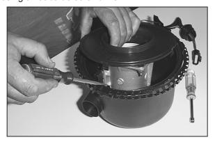
10. Using a flat blade screwdriver, push in and release the four clips that retain the mass air sensor retaining plate.
