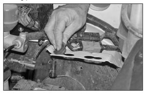
12. Remove the two air box mounting grommets from vehicle as shown.
