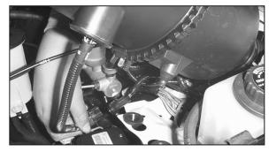
6. Disconnect the secondary mass air sensor electrical connection.
