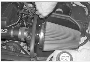
31. Install the Filtercharger onto the mass air sensor and secure it with the provided hose clamp.
