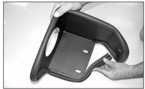
13. Install edge trim onto heat shield as shown. Trim if needed.
