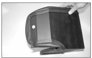
15. Install the provided "L" bracket (070952) onto heat shield as shown.
