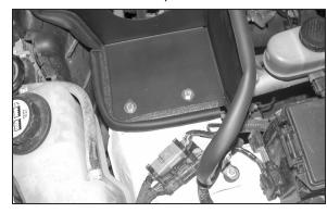
17a. On vehicles that did not come equipped with cruise control, install heat shield onto the vehicle, then secure with the provided hardware.
