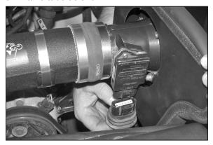
30. Reconnect the primary and secondary mass air electrical connection.
