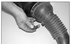
21. Remove the temp sensor from the stock intake tube as shown.
