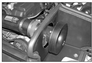
29. Install the mass air sensor assembly onto the new intake tube as shown.
