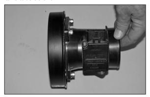
24. Attach the mass air adaptor to the mass air sensor using the gasket and provided hardware as shown.
