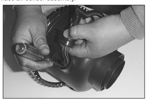
9. Slide the rubber grommet back and disconnect the primary mass air sensor electrical connection, using a flat balde screwdriver.
