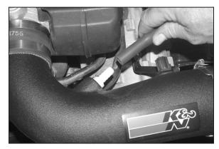
27. With the provided silicone hose reconnect the crank case vent to the new intake tube as shown.
