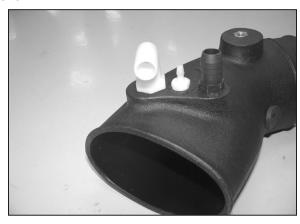
16. Install the provided vent fitting onto the new  $K\&N^{\circ}$  intake tube as shown.
