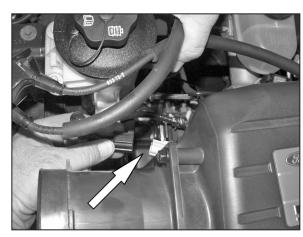
5. Disconnect the temp sensor electrical connection as snown.
