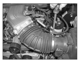
3. Loosen the hose clamp at the throttle body and mass air sensor as snown.
