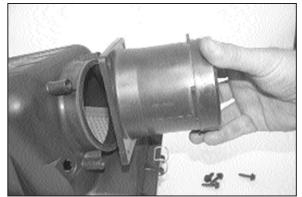
25. Remove the mass air sensor from the factory air box as shown.
