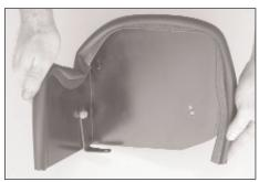
19. Install the edge trim onto the heatshield as shown. Trim if needed.
