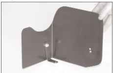
18. Install the bracket onto the heatshield as shown.
