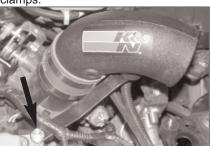
14. Install the new intake tube onto the throttle body, then mount the bracket onto the valve cover with the provided hardware.
