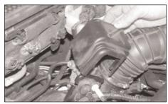
3. Pull up firmly to remove the throttle linkage cover as shown.
