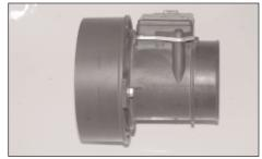
23. Bolt the mass air sensor onto the filter adaptor with the provided hardware as shown.
