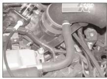
17. Reconnect the crank case vent with the provided silicone hose as shown.
