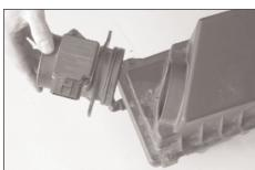
22. Unscrew the mass air sensor from the air box then remove the mass air sensor.
