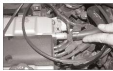
5. Disconnect the crank case vent hose from valve cover as shown.
