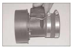
24. Install the silicone hose (08190) onto the mass air sensor with the provided hose clamp.
