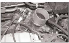
13. Install the silicone hose (08756) onto the throttle body with the provided hose clamps.
