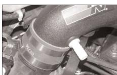
16. Install the hose mender onto the intake tube.
