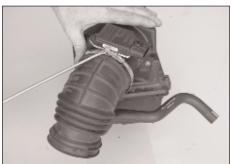
21. Remove clamp that secures the intake tube to the mass air sensor then remove
