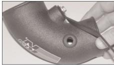
12. Install the provided grommet onto the intake tube as shown.
