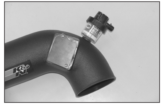
21b. On vehicles equipped with an air temperature sensor, install the mass air block off plate onto the K&N intake tube using the provided screws and spacers as shown.
