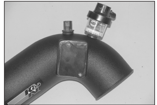
21d. On vehicles equipped with an air temperature sensor, install the factory grommet and air temperature sensor into the hole that was drilled in the previous step.
