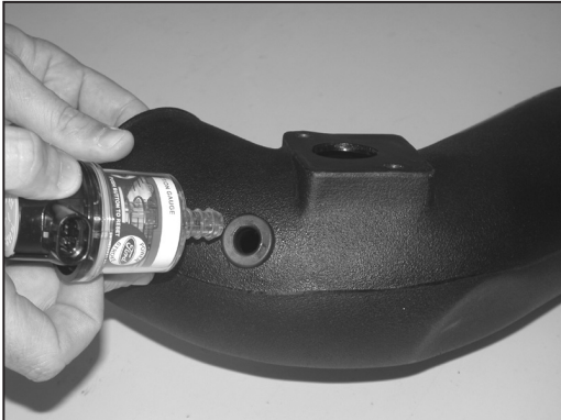
17. Install the factory grommet and restriction gauge into the K&N intake tube as shown.
