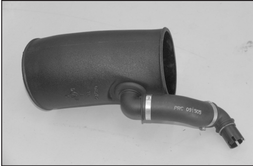
15d. On vehicles equipped with a one piece inlet tube and bellows, install the crank case vent tube assembly removed in step #15b into the grommet in the turbo inlet tube as shown.
