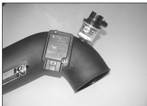
21. On vehicles equipped with a mass air sensor, install the mass air sensor into the K&N intake tube with the provided screws and spacers as shown.
