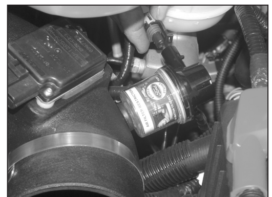
24. Reconnect the restrictor gauge electrical connection as shown.
