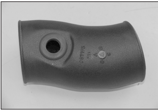
15c. On vehicles equipped with a one piece inlet tube and bellows, install the provided grommet into the turbo inlet tube as shown.
