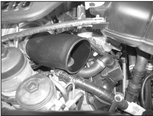
15e. On vehicles equipped with a one piece inlet tube and bellows, install the turbo inlet tube assembly onto the turbo. Rotate to align the crank case vent tube with the valve cover vent port. Snap the crank case vent tube into the valve cover vent port and secure the tube with the provided hose clamp.
