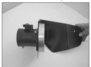
11. Assemble the filter adaptor and heat shield onto the mass air sensor as shown with the provided gaskets and hardware.
