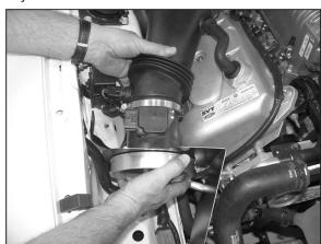
16. Install the mass air assembly onto the intake tube.
