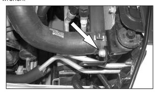
14. Install the provided bracket onto the radiator using the bolt that was removed in the previous step.
