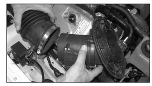
7. Disconnect the mass air from intake tube as shown.
