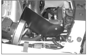
17. Connect the heatshield onto the "L" bracket as
