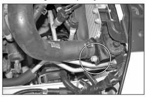
13. Remove the radiator mount bolt with a 13mm wrench.
