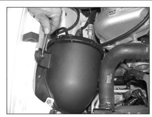
9. Loosen and remove the bolt that retains the air filter assembly onto the vehicle as shown.
