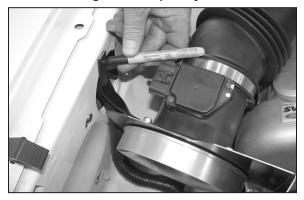
18. Align the bracket to the inner fender then mark the fender with a felt pen.
