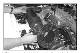
5. Release the intake tube at the throttle body then lift complete intake track up to access the mass air electrial connection.
