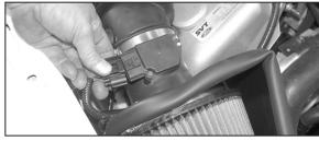
23. Reconnect the mass air electrial connection as shown.
