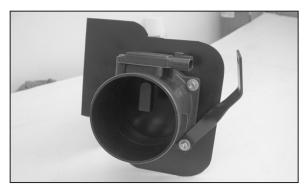
12. Install the provided bracket onto the mass air assembly with the 6mm x 25mm allen bolt as shown
