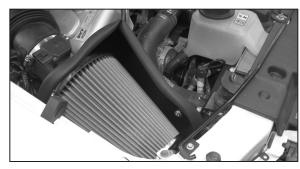
22. Reinstall the mass air assembly onto the intake tube and secure the brackets with the provided sheet metal screw and 6mm bolt onto the "L" bracket.
