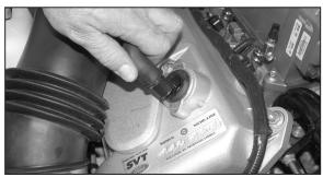
4. Remove crank case vent hose from valve cover as shown.
