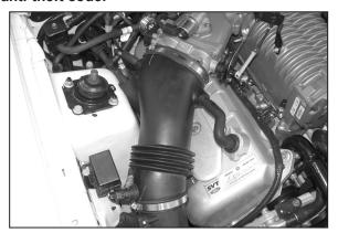
2. Loosen the hose clamps at the throttle body and mass air.
