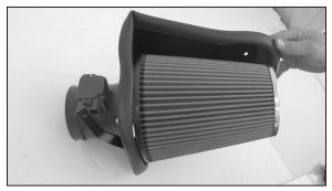
21. Install the filter charger onto the mass air assembly and secure it with the provided hose
