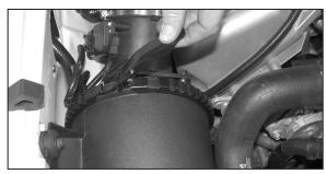
3. Release the filter clam shell clamp as shown.
