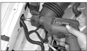
19. Remove the mass air assembly from the vehicle and using a 3/16 drill bit, drill out the marks.
