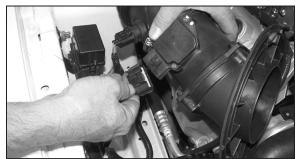
6. Disconnect the mass air electrial connection.
