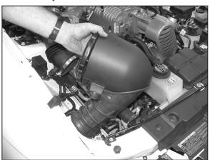
10. Pull the air filter assembly upward and remove from vehicle.
