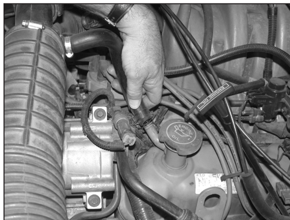
4. Loosen the hose clamp that secures the crank case vent to the valve cover then remove hose.
