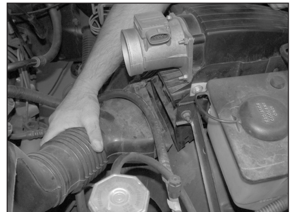
6. Remove the fresh air intake tube from the bottom of air box as shown.
