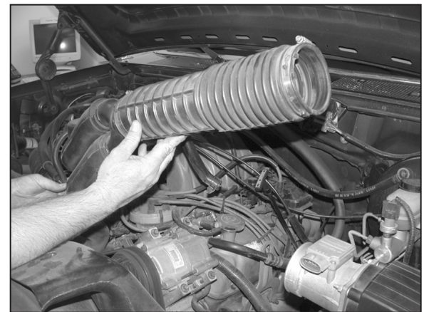
5. Loosen the three hose clamps that secure the intake tube to the air box and throttle body then remove the intake tube.
